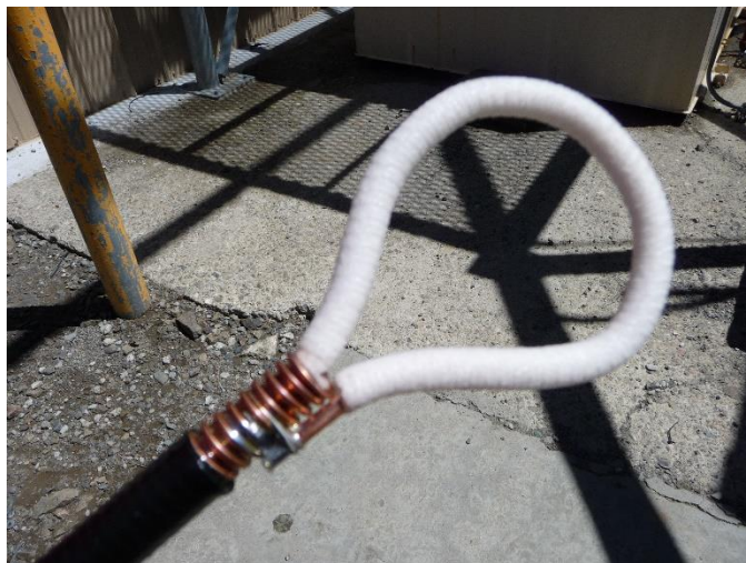
Figure 3 – Loop Antenna Used as RF Probe When Seeking & Measuring PIM Noise Energy on Tower
