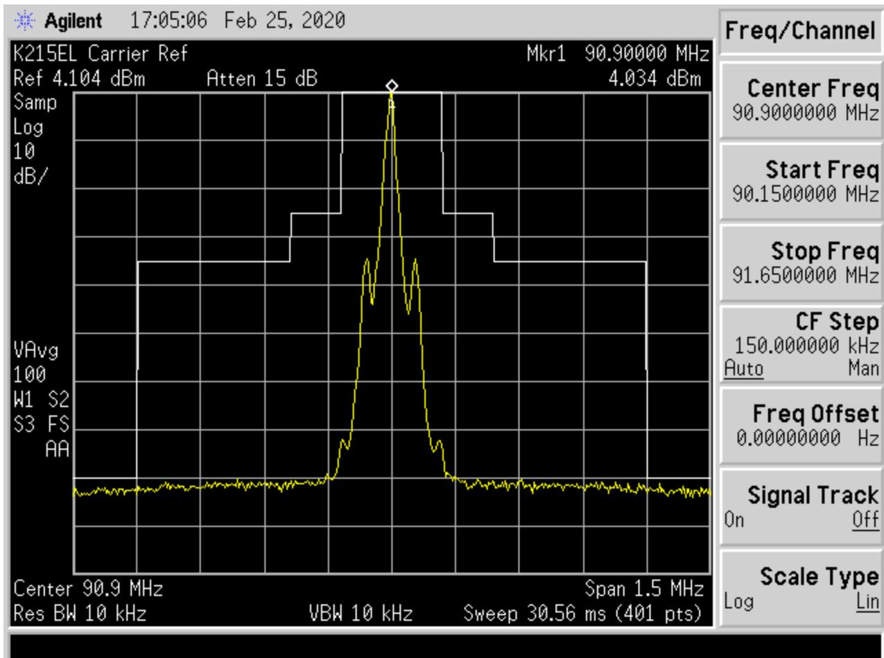
Item 2 – Fully modulated monophonic carrier with RDS, shown within mask limits.
