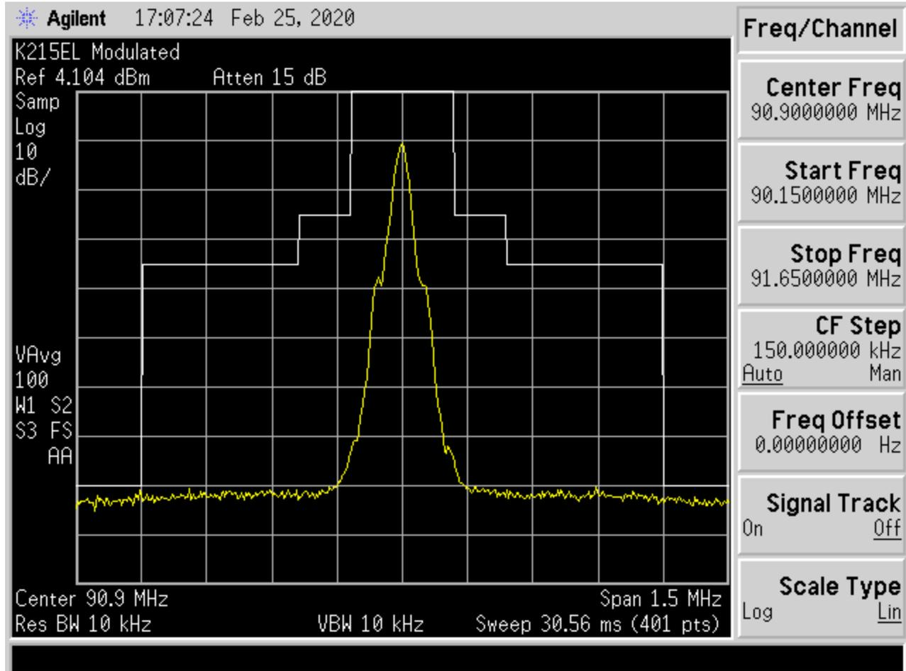
Item 3 – Upper third order inter-modulation product of K215EL and KZMU measured from the common transmission line to the common 2 bay antenna, via directional coupler.
