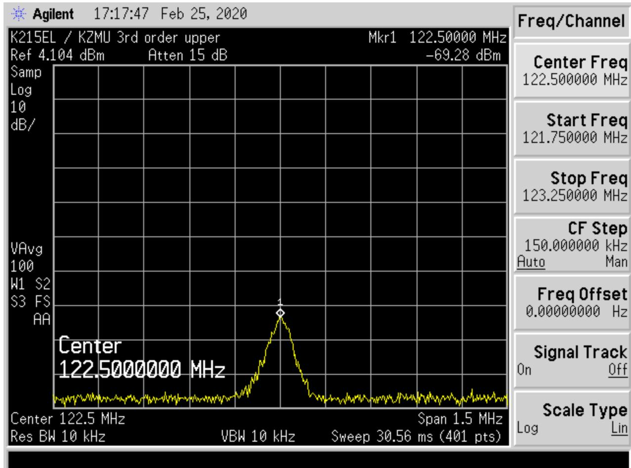
Item 4 - Lower third order inter-modulation product of K215EL and KZMU measured from the common transmission line to the common 2 bay antenna, via directional coupler.
