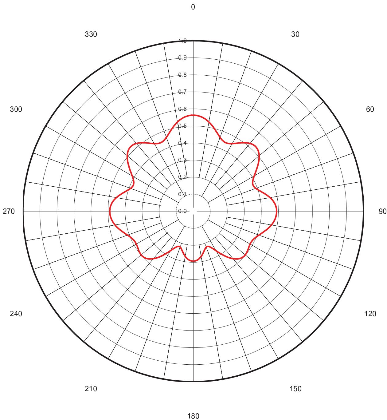
**TABULATION OF AZIMUTH PATTERN/VERTICAL POLARIZATION**Azimuth Pattern Drawing #: **TUMLP-SP4V-6050**
