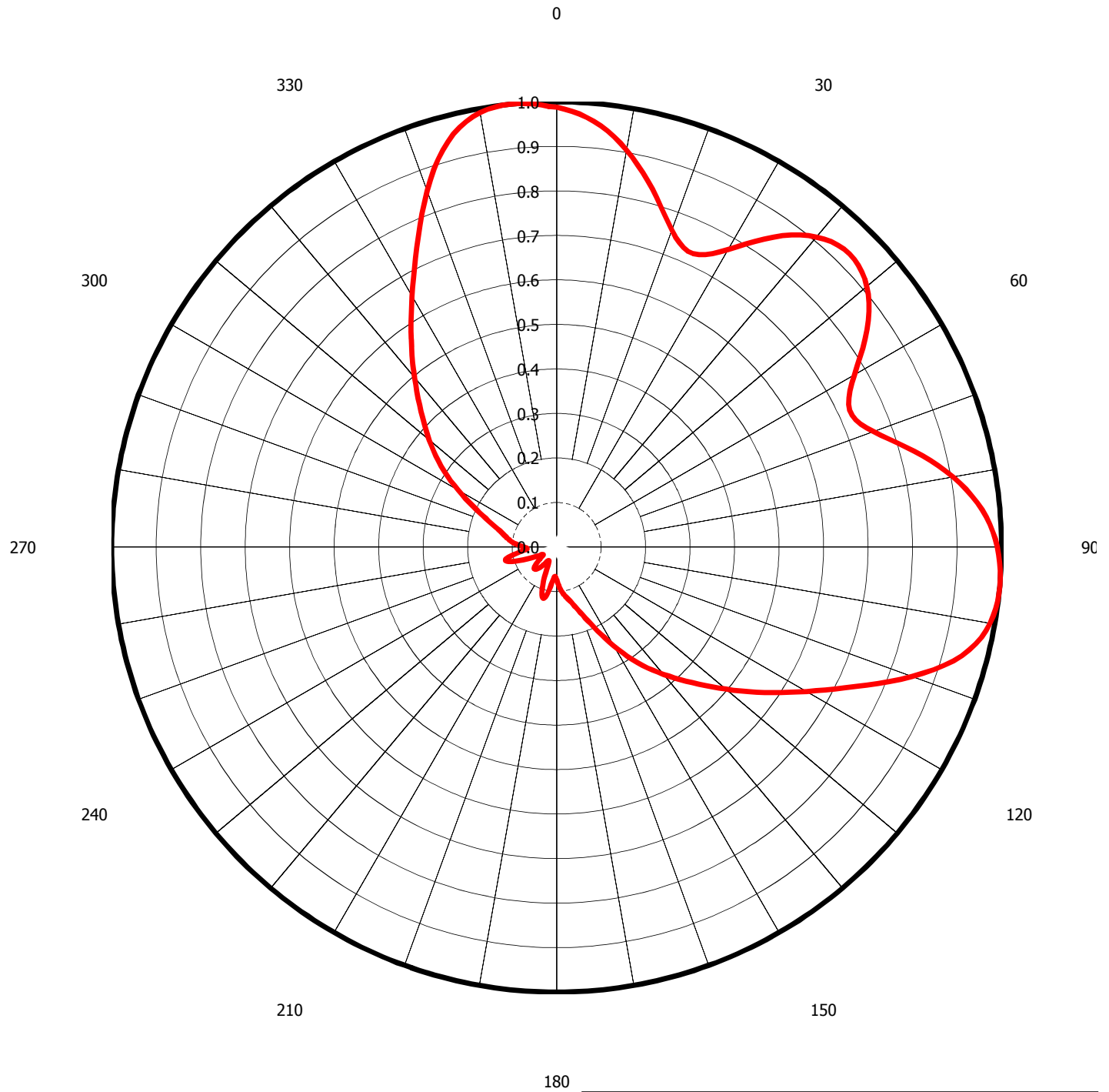
Figure 1 STA Antenna Azimuthal Pattern W21DB-D Meridian, MS Facility ID 185229 Ch. 21 (digital) 0.005 kW
