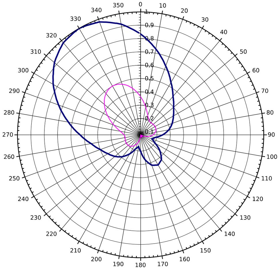
Blue plot shows azimuth pattern relative field for horizontal polarization
