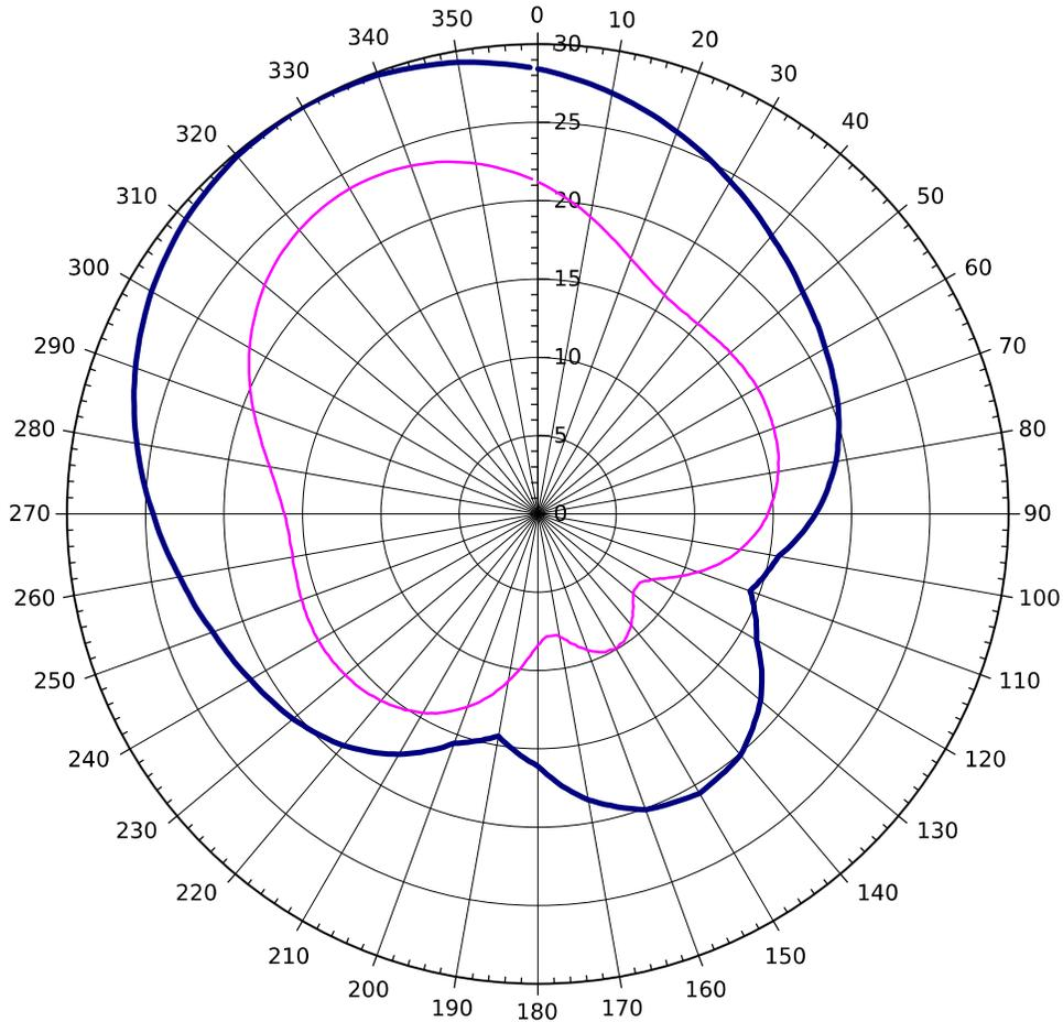
Blue plot shows effective radiated power (dBk) for horizontal polarization
