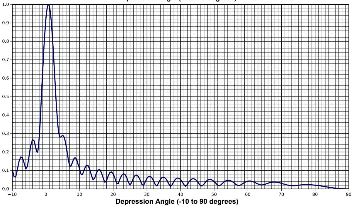
ELEVATION PATTERN Dielectric TFU-17ETT/VP-R S340
