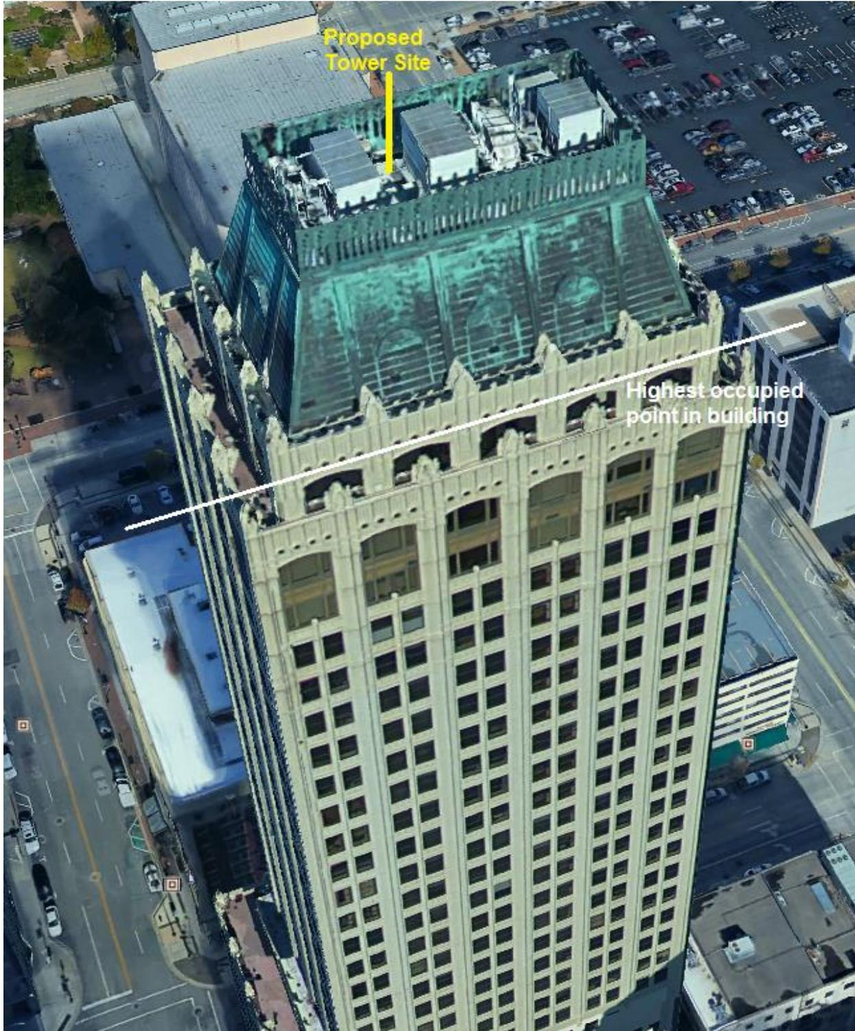
Yellow line does not represent the scale of the tower height. Since the interfering contour of the proposed station is less than 2 meters, the interference will not even leave the mounting pole.
