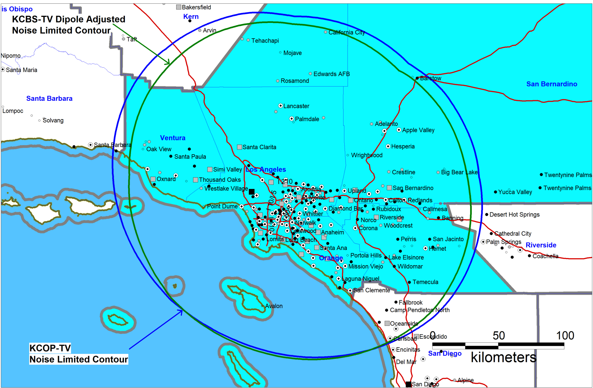
Coverage Contour Comparison KCOP-TV Licensed Ch 13 Los Angeles, CA ERP 120 kW HAAT 904 m Directional Antenna ATSC 1.0 Host KCBS-TV Licensed Ch 31 Los Angeles, CA ERP 485 kW HAAT 1,095.0 m Directional Antenna
