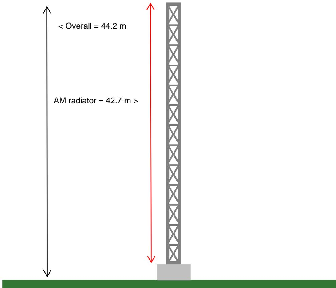
WKPT replacement tower will be a uniform cross section guyed steel tower 145 feet (44.2 meters) overall. The radiator will be 140 feet (42.7 meters) and will utilize the existing 1/4 wavelength ground system resulting in an efficiency of 293.9 mV/m/km/kW.
