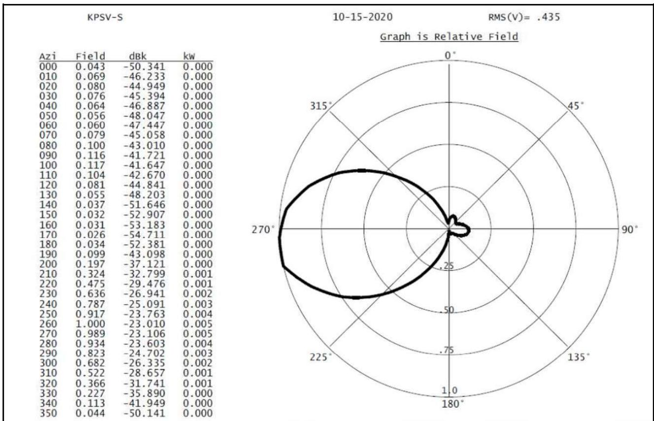
Antenna rotated to 260 degrees at 5 watts ERP
