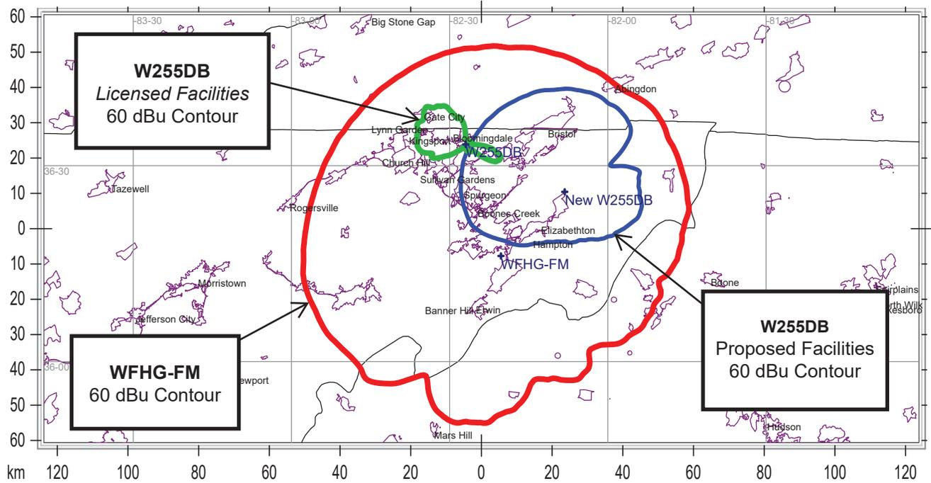
FM Translator Station W255DB will rebroadcast Station WFHG-FM at Bluff City, Tennessee. The service contour of W255DB with the proposed facilities will not exceed the 1.0 mV/m (60 dBu) contour of WFHG-FM. WFHG-FM co-owned with W255DB by Bristol Broadcasting Company, Inc.
