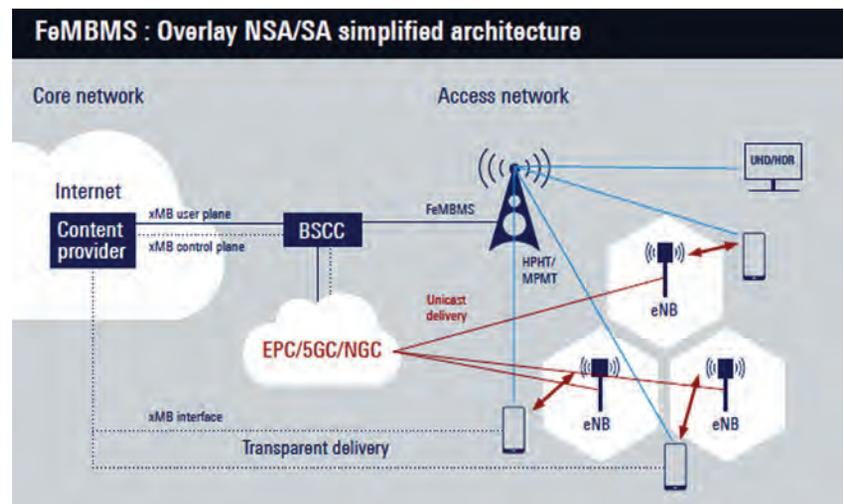
Figure 3. 5G Broadcast overlay NSA/SA simplified architecture.
