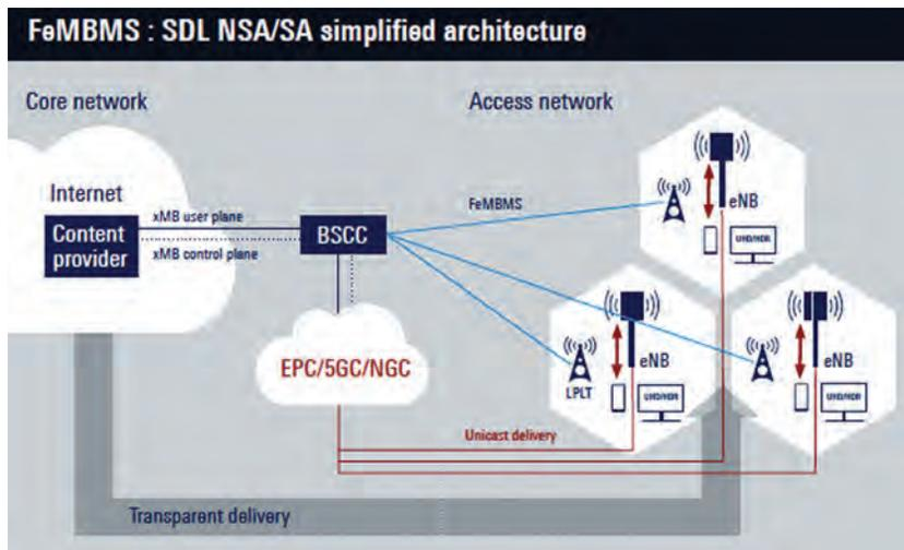
Figure 4. 5G Broadcast SDL NSA/SA simplified architecture.
