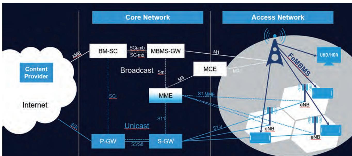
Figure 1. 5G Broadcast overall architecture.
