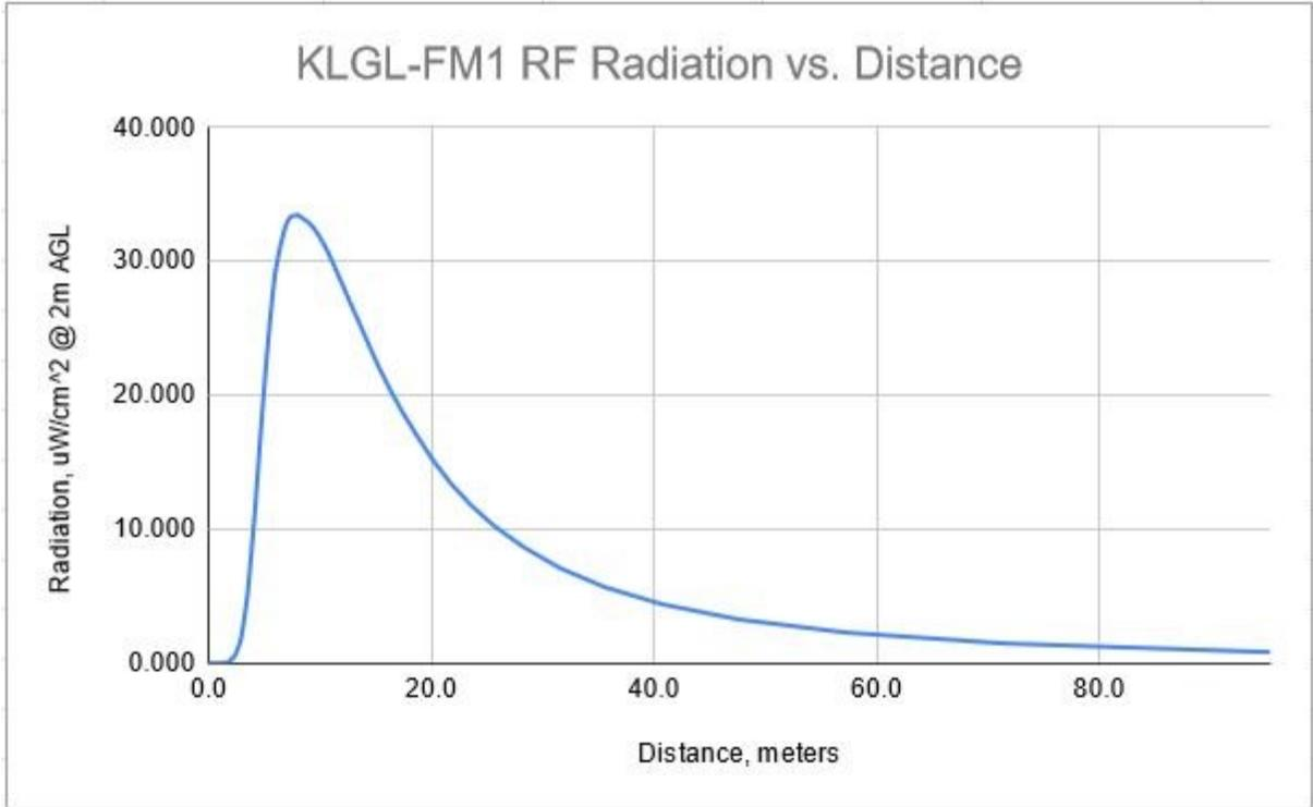
Maximum Radiation is  $33.5\mu\text{W}/\text{cm}^2$  at 8.0m from the tower base
