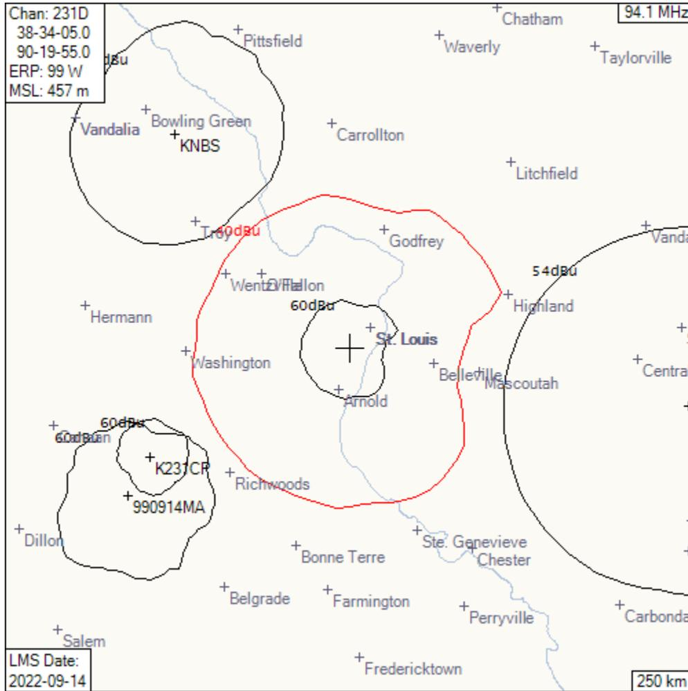
The proposed 40 dBu f(50,10) contour does not overlap any of the protected 60 dBu f(50,50) contours.
