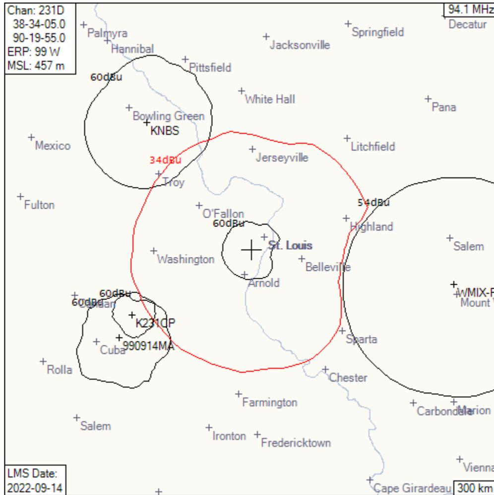
There is no overlap between the proposed 34 dBu f(50,10) contour and the protected WMIX-FM 54 dBu f(50,50) contour.
