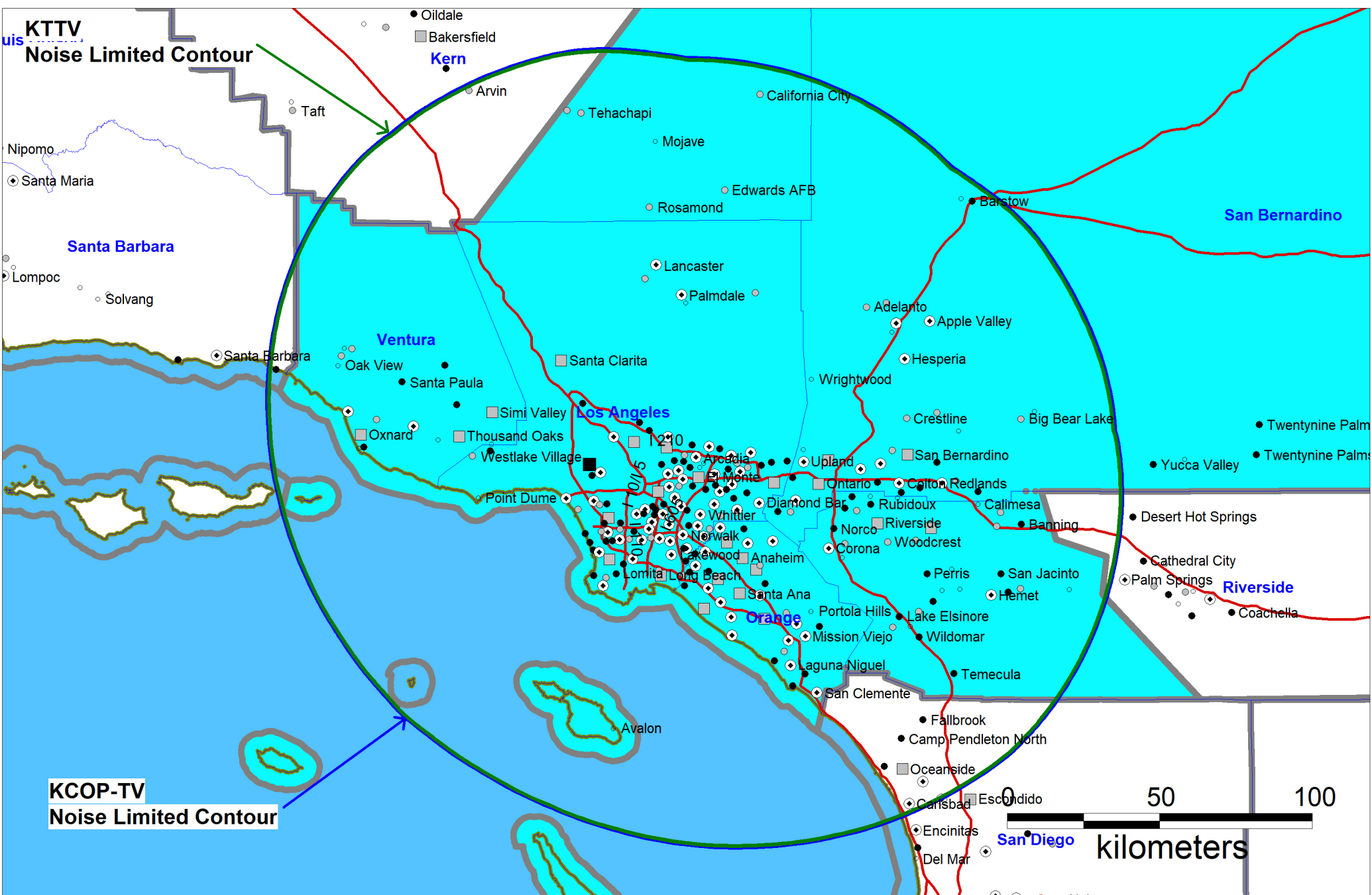
Coverage Contour Comparison KCOP-TV Licensed Ch 13 Los Angeles, CA ERP 120 kW HAAT 904 m Directional Antenna ATSC 1.0 Host KTTV Licensed Ch 11 Los Angeles, CA ERP 115 kW HAAT 902 m Directional Antenna
