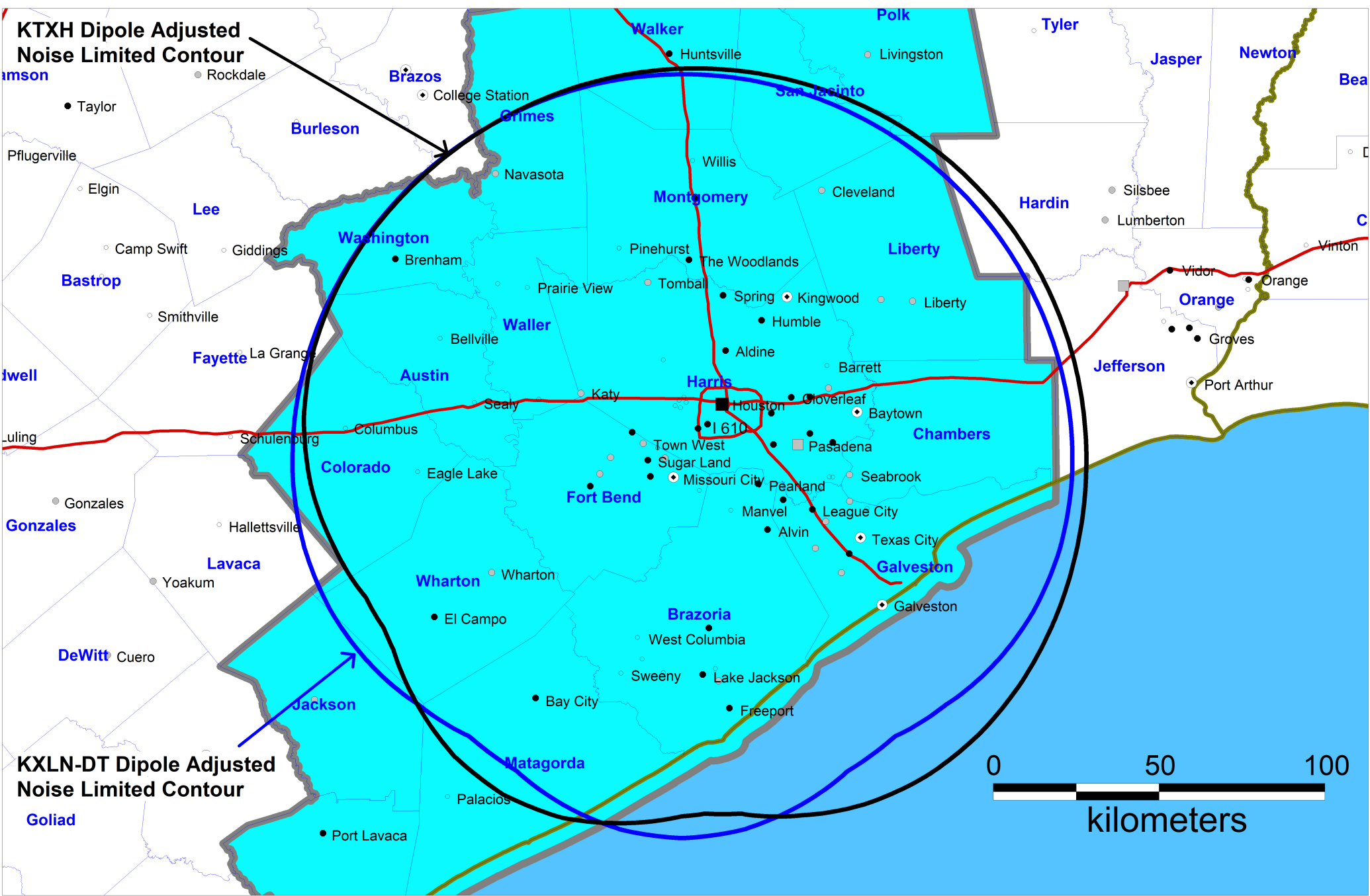
Coverage Contour Comparison KTXH Licensed Ch 19 Houston, TX ERP 1,000 kW HAAT 595 m Directional Antenna ATSC 1.0 Host KXLN-DT Licensed Ch 30 Rosenberg, TX ERP 1,000 kW HAAT 592 m Directional Antenna
