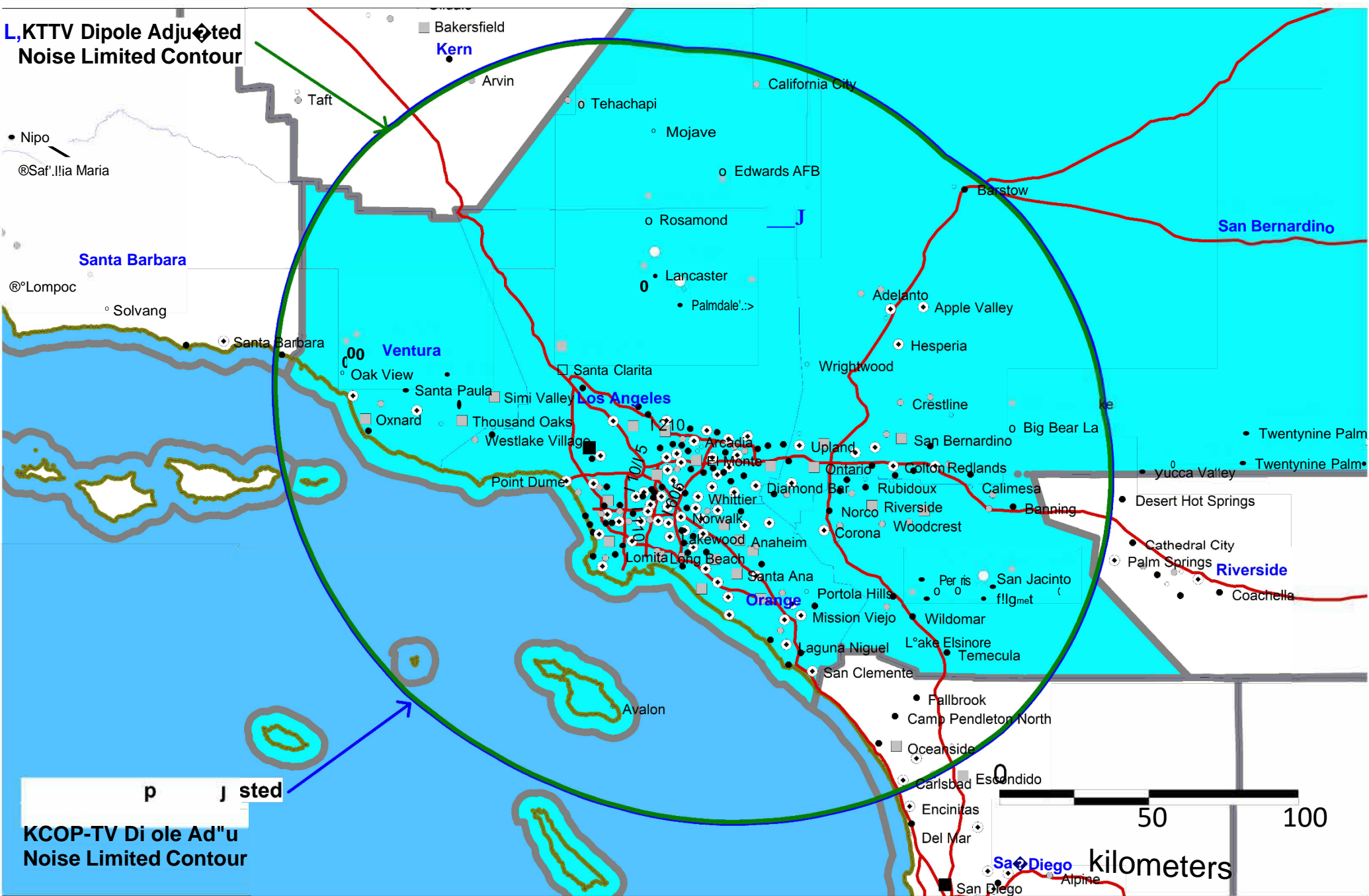
FCoverage Contour Comparison KCOP-TV Licensed Ch 13 Los Angeles, CA ERP 120 kW HAAT 904 m Directional Antenna KTTV Licensed Ch 11 Los Angeles, CA ERP 115 kW HAAT 903 m Directional Antenna
