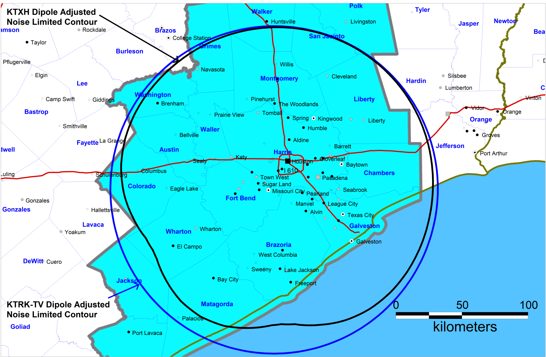
Coverage Contour Comparison KTXH Licensed Ch 19 Houston, TX ERP 1,000 kW HAAT 595 m Directional Antenna ATSC 1.0 Host KTRK-TV Licensed Ch 13 Houston, TX ERP 32.4 kW HAAT 588 m OMNI
