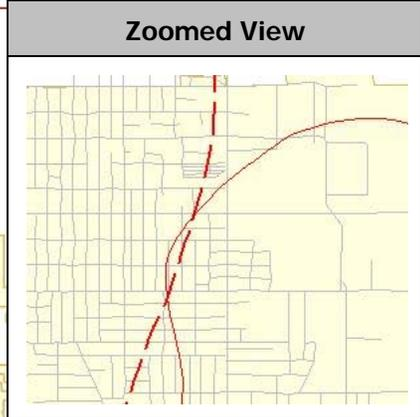
Note: The FM Translator station's originally proposed 60 dBu contour is shown below as the thin red contour. The 60 dBu contour of the facility proposed herein is the thick red dashed contour. Because these contours overlap, the instant proposal is considered a minor change.
