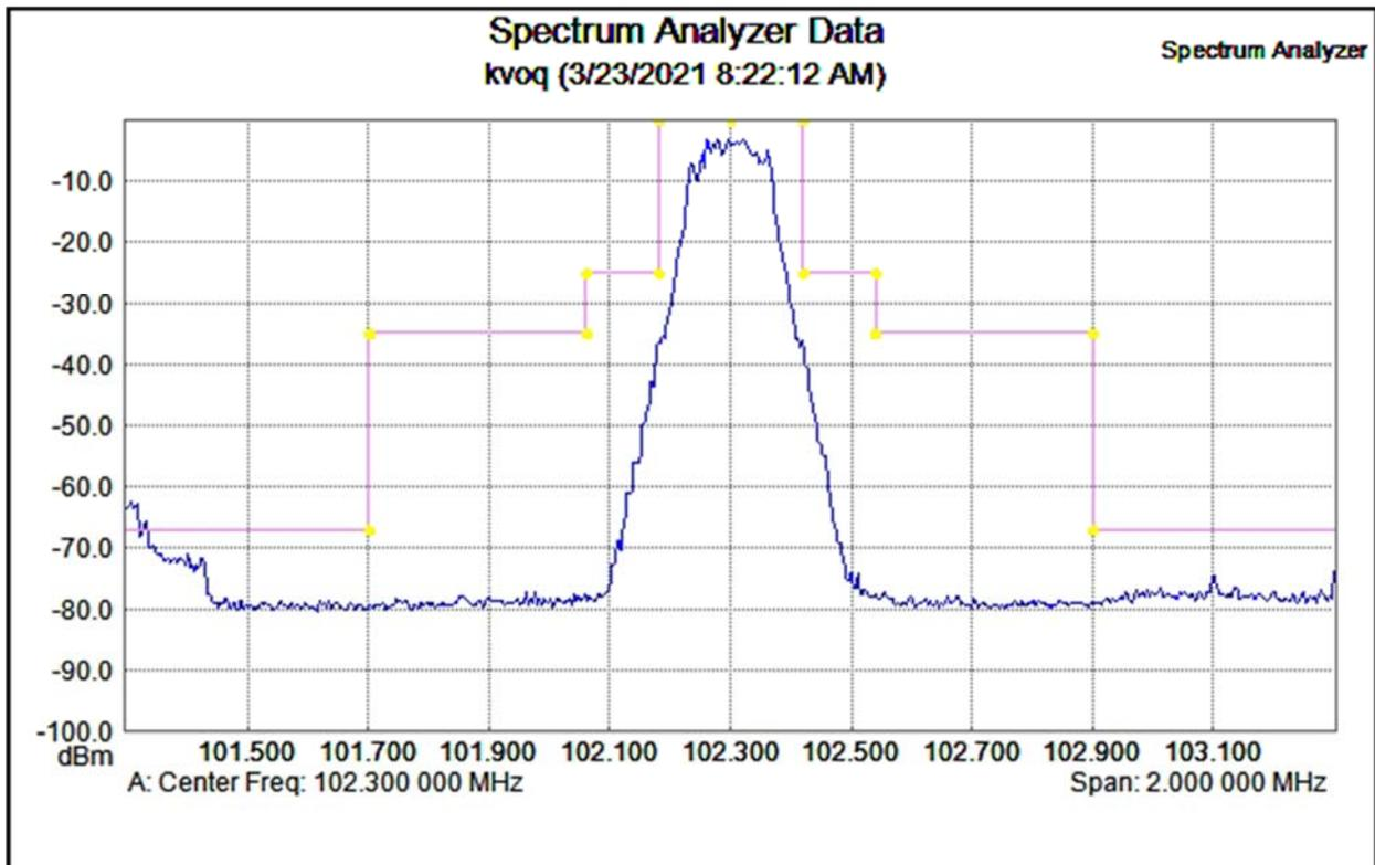
An Intermod product was produced on 101.1MHz from significant incoming power from KRFX on 103.5MHz on the combiner. This signal at 101.1MHz was 55db below the carrier at the input to the combiner. **The combiner input filter attenuation at 101.1MHz is 38 db so the intermod product from KVOQ at the combiner output should be more than 80db below carrier.** Significant incoming signal from KOSI at 101.1 MHz prevented actual measurement of the intermod product on the output of the combiner.
