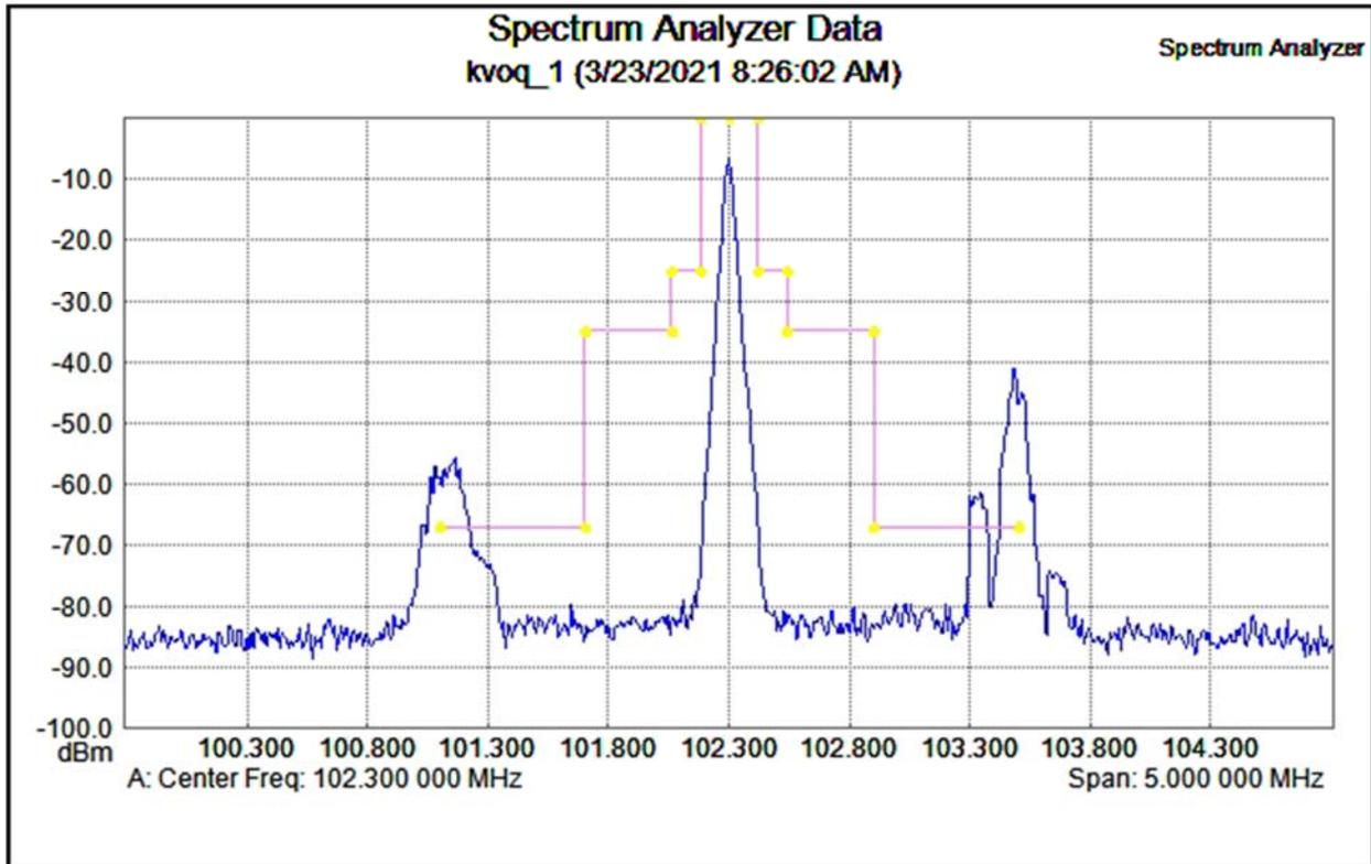
All other intermod products were measured at the output of the combiner. All other intermod products were measured more than 67 dB below carrier level.
