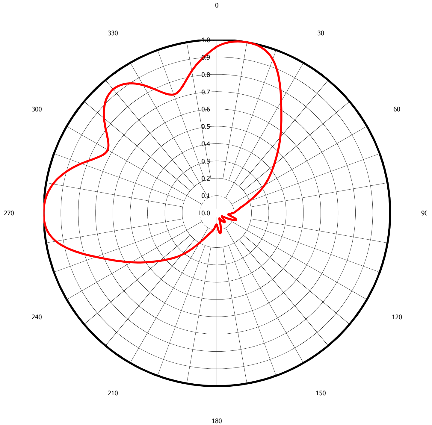
Figure 1 Antenna Azimuthal Pattern KNXG-LD College Station, TX Facility ID 182059 Ch. 27 2.4 kW Directional
