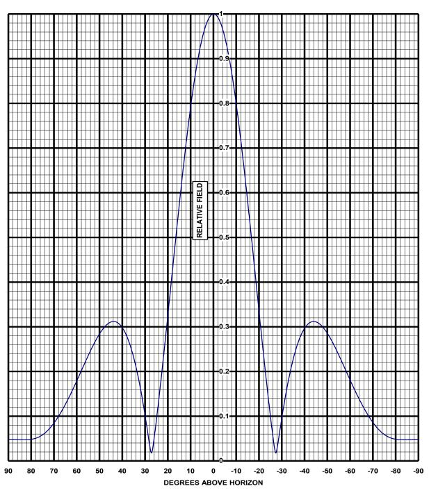
Model: JUHD Description: UHF Panel Antenna -0 ° Beam Tilt, 0% Null Fill
