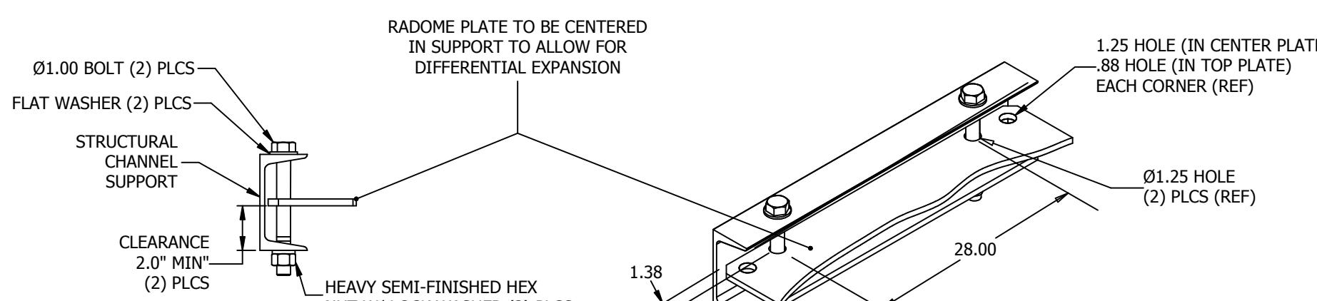
NOTE: POSSIBLE MOUNTING FOR TOP PLATE AND CENTER PLATES TO HORIZONTAL SUPPORTS
