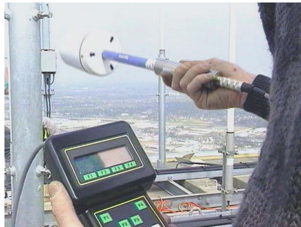
Figure 6. RF field measurements are routinely performed with broadband RF field probes and meters, as above, whenever changes in the operational environment occur.
