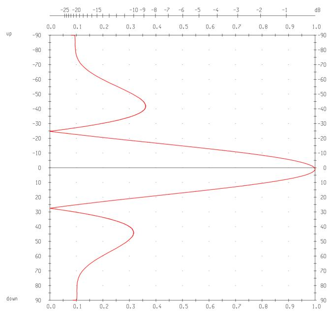
frequency in MHz 213.000 azimut in 305.0 omni-dir in dBd 4.08
