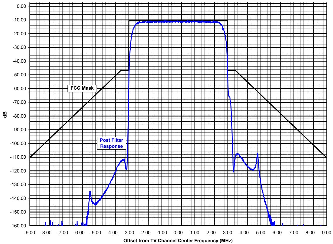
Blue: Total Response of a 12-Section Filter plus transmitter exciter and power amplifiers
