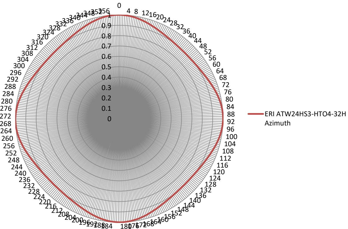
Figure 1 – ERI ATW24HS3-HTO4-32H Azimuth Pattern in Relative Field Values
