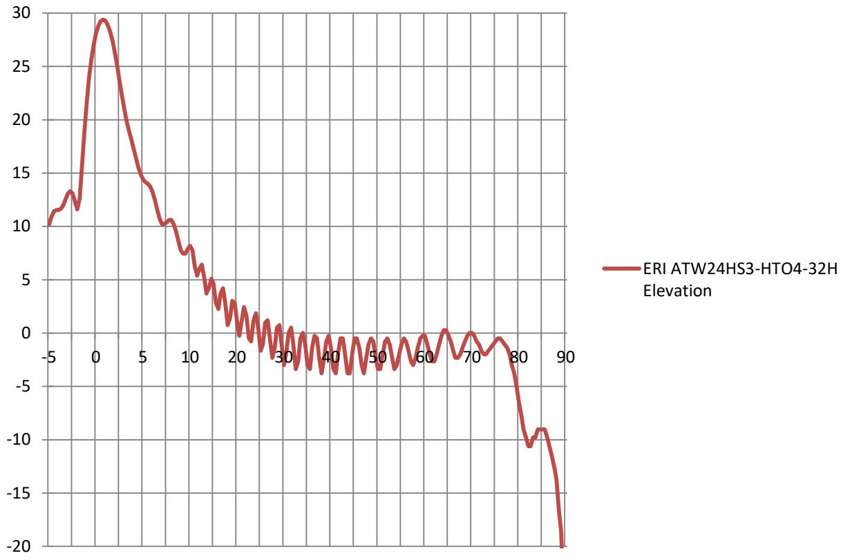
Figure 4 – ERI ATW24HS3-HTO4-32H Elevation Pattern Power in dBk Values
