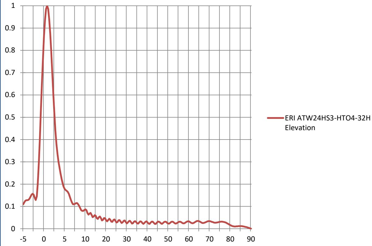
Figure 3 – ERI ATW24HS3-HTO4-32H Elevation Pattern in Relative Field Values
