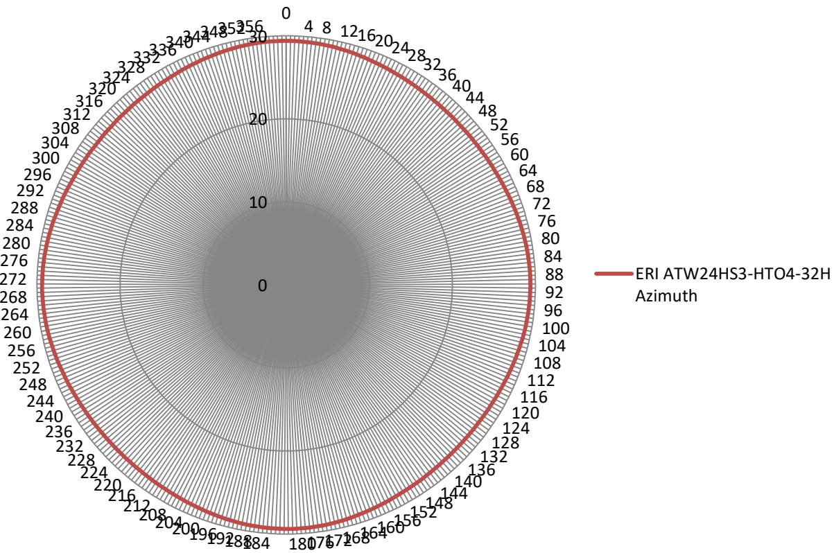
Figure 2 – ERI ATW24HS3-HTO4-32H Azimuth Pattern Power in dBk Values
