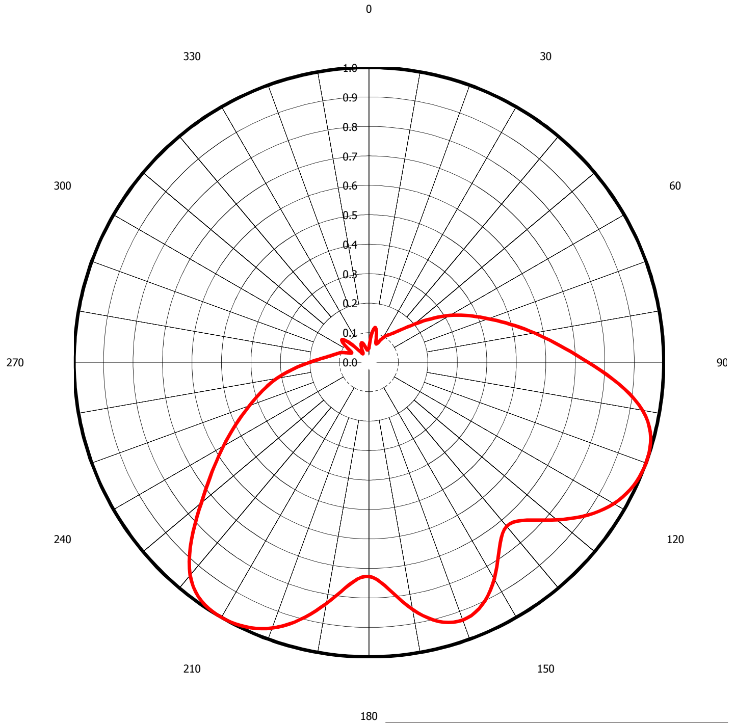
Figure 1 Antenna Azimuthal Pattern K31LQ-D Sherman, TX Facility ID 184857 Ch. 31 (digital) 4.8 kW
