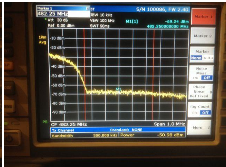
Lower and Upper Adjacent Channel Measurement Photos indicating Shoulder Amplitude Level
