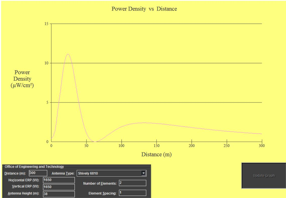
Maximum:  $11.15 \mu\text{W}/\text{cm}^2$  @ 24m horizontal distance from tower (12m above ground level)
