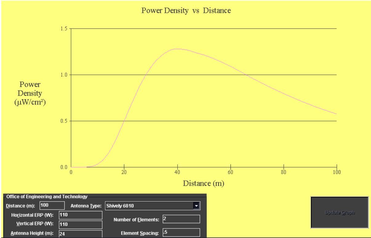
Maximum: 1.3  $\mu\text{W}/\text{cm}^2$  @ 40m horizontal distance from tower (12m above ground level)
