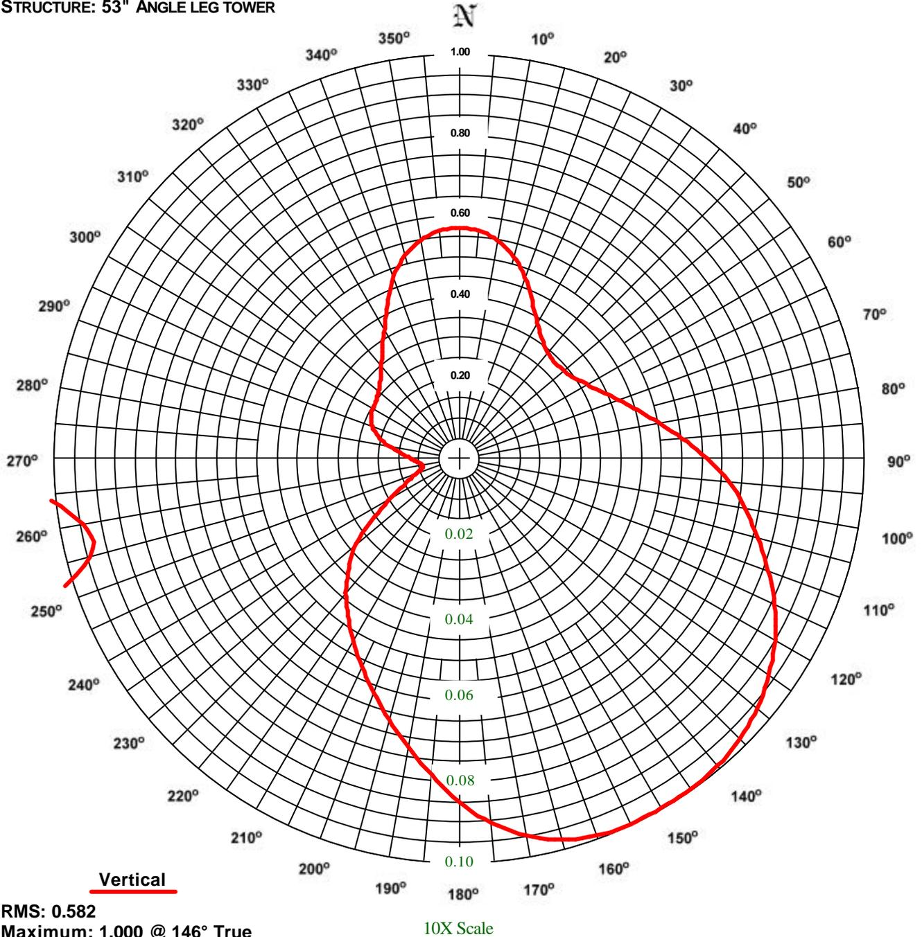
COMMENTS: MEASURED PATTERN OF THE VERTICAL COMPONENT. COMPOSITE PATTERN: THIS PATTERN SHOWS THE MAXIMUM OF EITHER THE VERTICAL AZIMUTH VALUES. THIS PATTERN IS GREATER THAT 85% OF THE FCC FILED COMPOSITE PATTERN BMPED-20050202AFK
