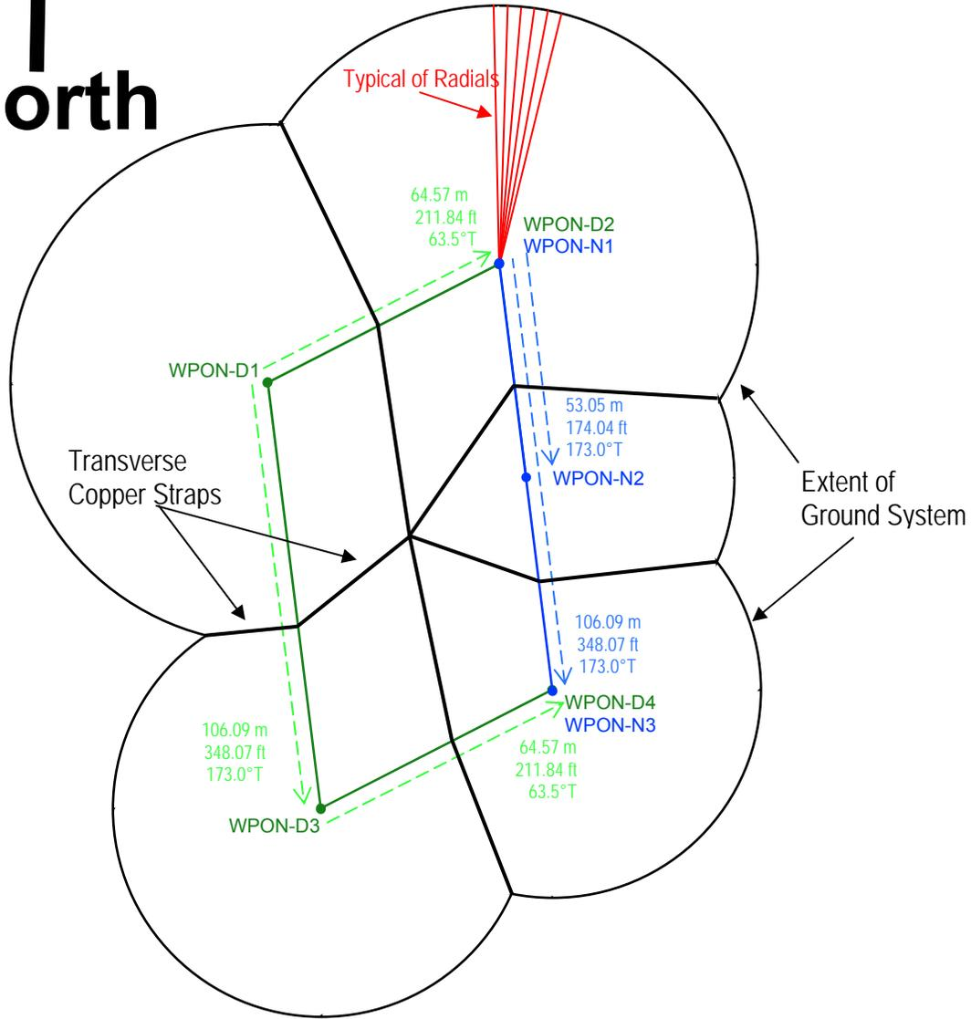
The proposed ground system will consist of 120 buried copper radials, extending 64.6 meters (212 feet) in length, about the base of the Daytime Towers 1 and 2 and 51.3 meters (168 ft) in length around the remaining daytime and nighttime towers. Radials will run the entire length except where shortened to terminate at property boundaries or at transverse copper straps running midway between the towers. The material used for the radial will be #10 AWG, soft drawn copper wire.
