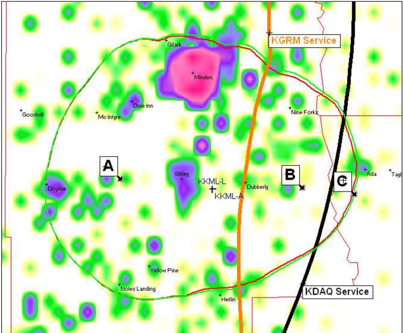
KKML (FM) coverage (license in red, proposed changes in green) showing the proposed 60dbu (green contour) is the same or slightly larger than that of the licensed red contour. There is a less than 0.25% shrinkage around the pattern (about 1 square kilometer across western half or Zone "A") in addition to the slight increase (Zone "C") in area and population to the east. This expansion is of no consequence as the station's expansion in Zone "B" is third service (forth counting recent KLHV)
