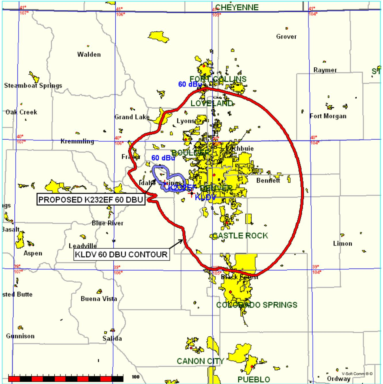
FIGURE 6, PRESENT AND PROPOSED 60 DBU CONTOURS
