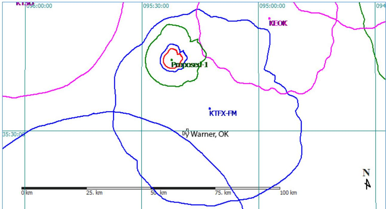
The green contours represent co-channel interfering (40 dBu) to co-channel protected (60 dBu) contours. Blue contours represent first-adjacent channel interfering (54 dBu) to first-adjacent protected (60 dBu) contours. Magenta contours represent second and third-adjacent channel interfering (100 dBu) to second and third-adjacent protected (60 dBu) contours. Red contours represent co-channel protected (60 dBu) to co-channel interfering (40 dBu) contours.
