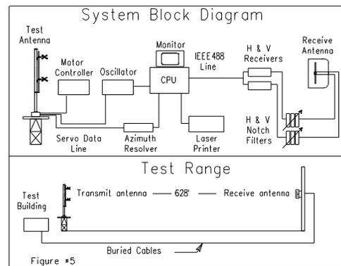
The antenna under test was operated in the transmitting mode and fed from a HP8657D signal generator. The frequency of the signal source was set at 88.9 MHz and was constantly monitored by a Rohde & Schwarz ESVD measuring receiver.
