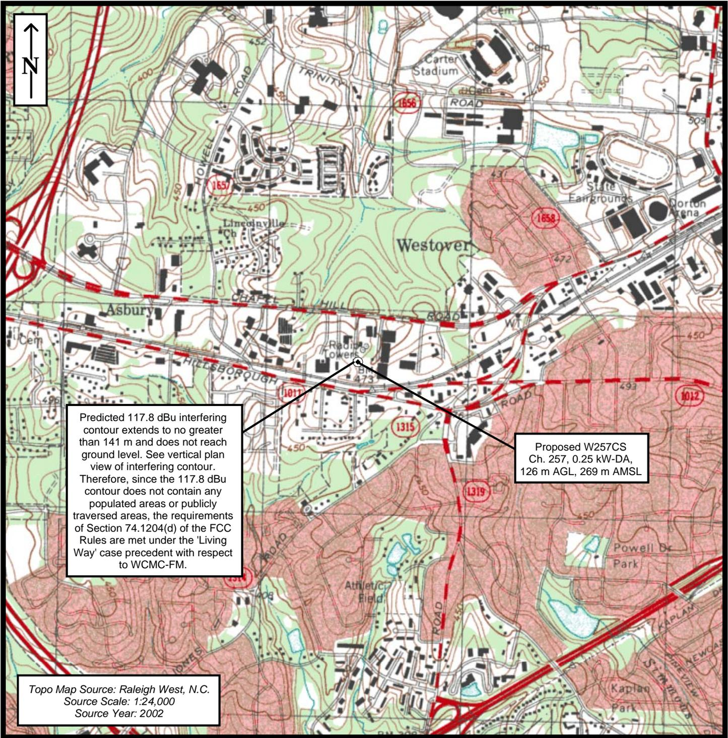
Predicted 117.8 dBu interfering contour extends to no greater than 141 m and does not reach ground level. See vertical plan view of interfering contour. Therefore, since the 117.8 dBu contour does not contain any populated areas or publicly traversed areas, the requirements of Section 74.1204(d) of the FCC Rules are met under the 'Living Way' case precedent with respect to WCMC-FM.
