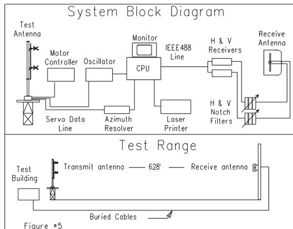
and a US Digital angle position indicator. The resolution of this angle position indicator is one-hundredth of a degree.
