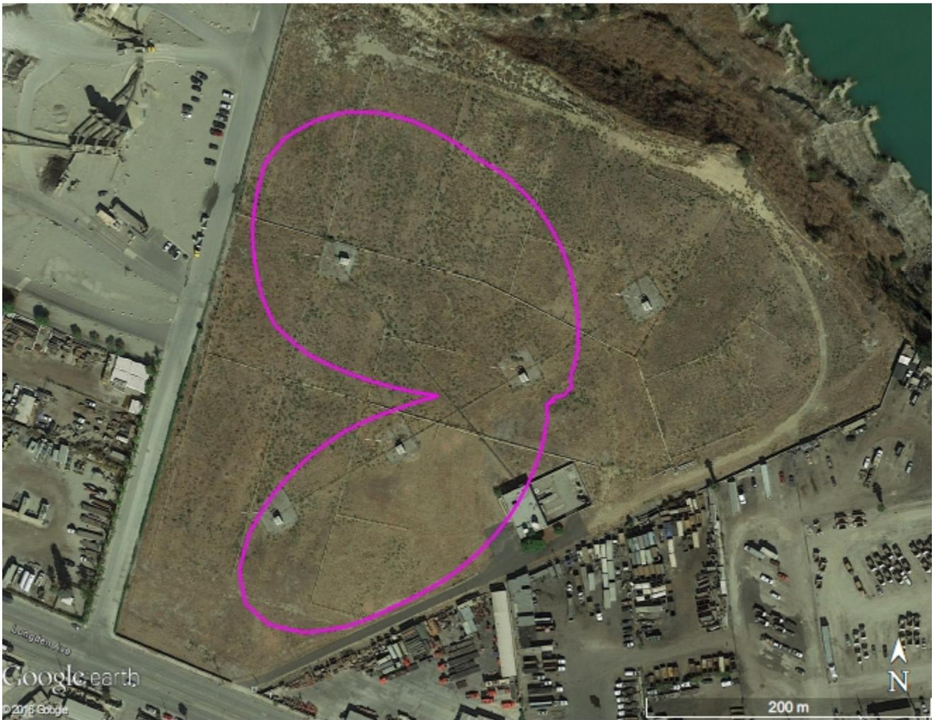
*The 116dBu contour is contained within the boundary of the KDIS Tower site.*
