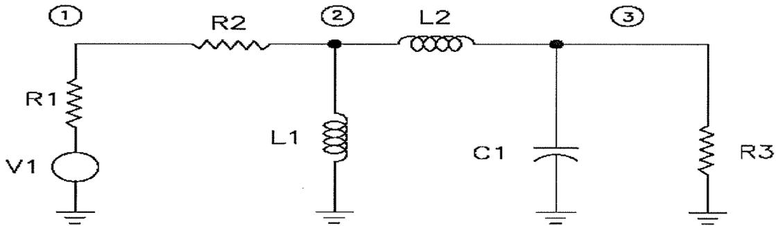
The above circuit was analyzed with the Engineering Circuit Analysis program (ECA) for each Tower. Resistors R1 (100k  $\Omega$ ) and R2 (0.1  $\Omega$ ) were located in the circuit for measurement locations of impedance and current.
