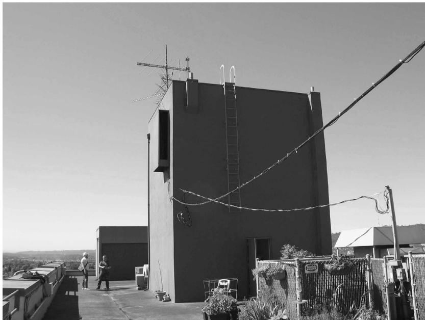
At normal roof level, 8.1 m lower than the penthouse roof, a maximum level of  $18.9 \mu\text{W}/\text{cm}^2$  at 3.22 m was calculated, equating to 9.4% of the uncontrolled MPE.
