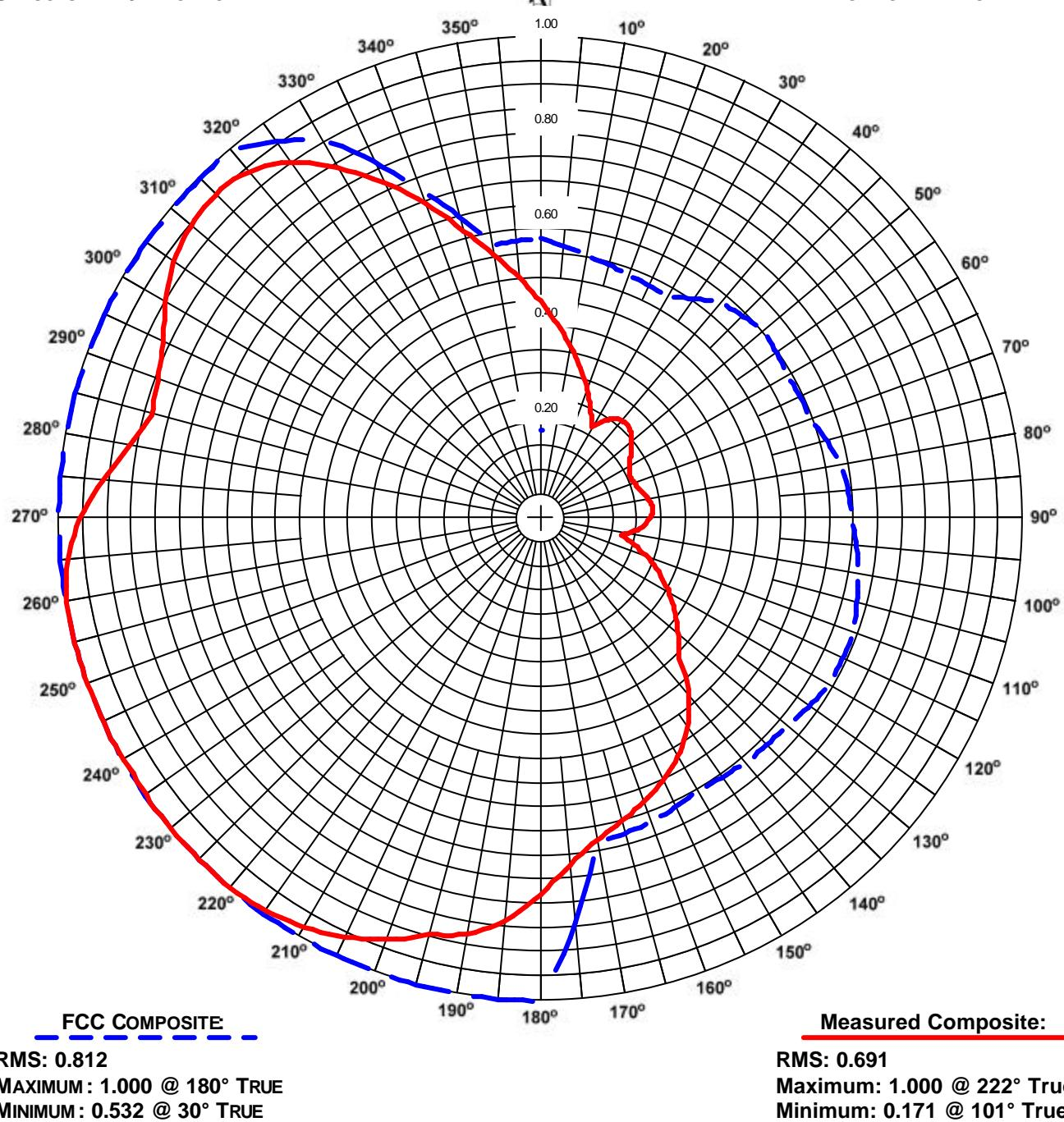
COMMENTS: COMPOSITE PATTERN: THIS PATTERN SHOWS THE MAXIMUM OF EITHER THE H OR V AZIMUTH VALUES. THIS PATTERN IS GREATER THAT 85% OF THE FCC FILED COMPOSITE PATTERN BPED-20031106AAJ
