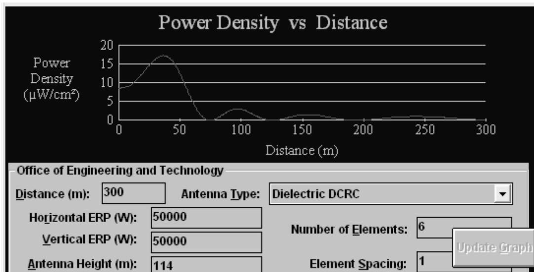
The Max Power Density was found to be 17.1659055228049  $\mu\text{W}/\text{cm}^2$  at 36 meters.
