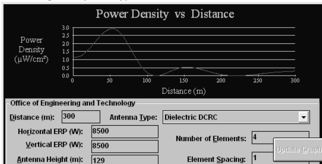
The Max Power Density was found to be 2.92767686849758  $\mu\text{W}/\text{cm}^2$  at 52.8 meters.
