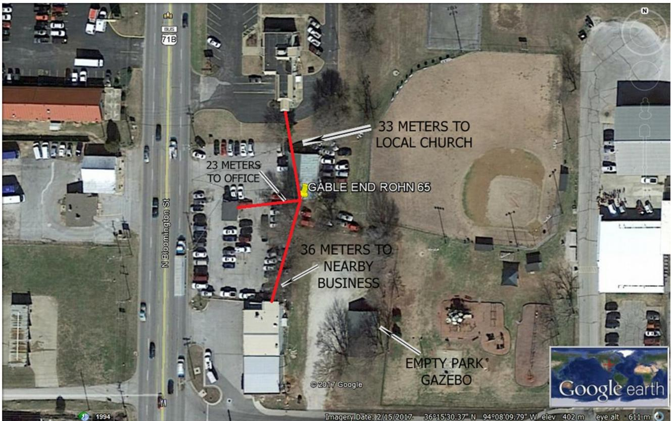
Any potential listener in the used car lot outside and next to the small office / storage building would receive an interfering contour of 112.8dBu or less from KENJ-LP
