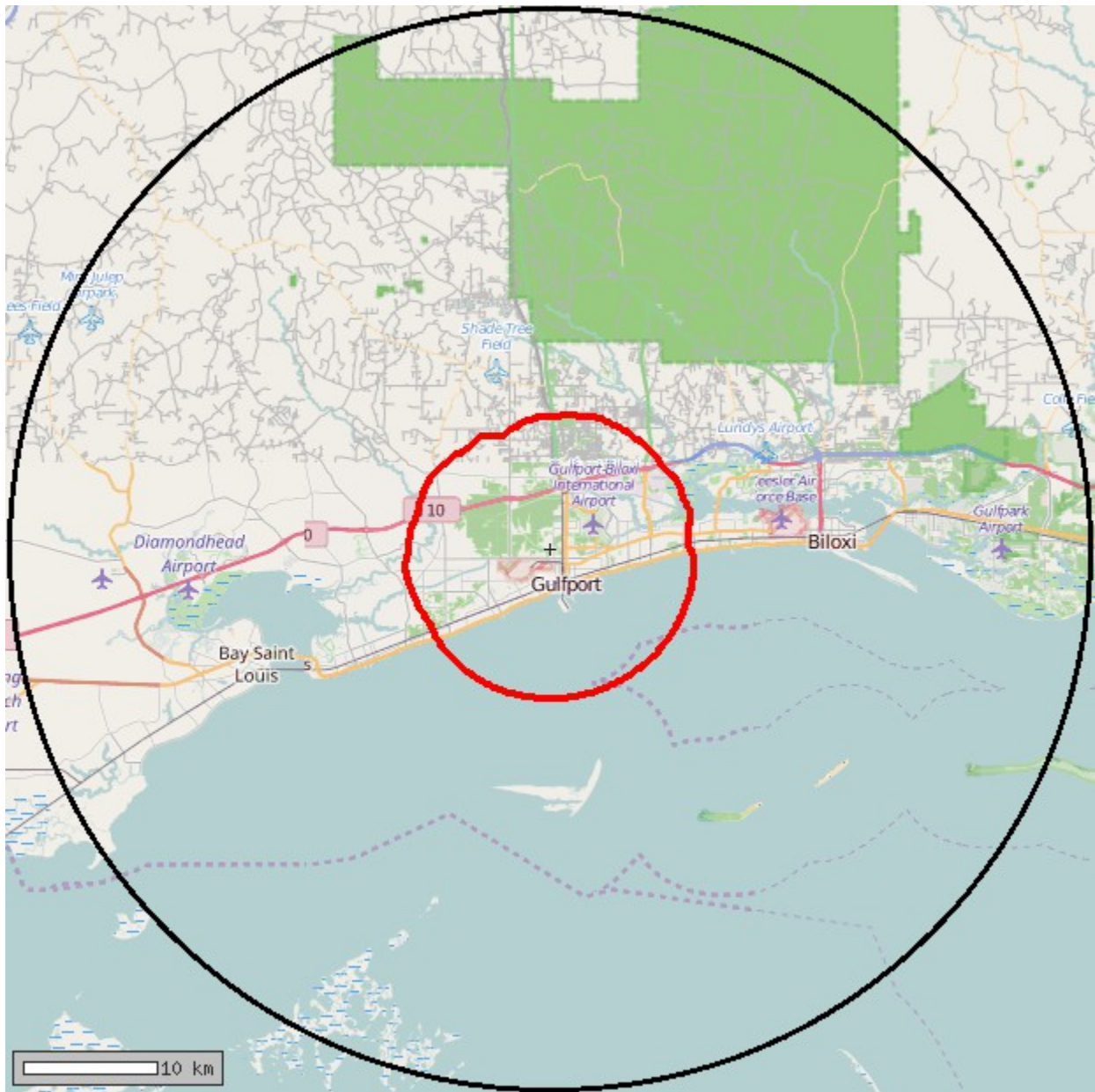
Figure 1 : The map above depicts the F(50,50) 60 dBu contour of the proposed fill-in translator (red contour) and a circle with a radius of 25 miles extending from the WQFX 1130 AM (primary station, Facility ID 61306, black contour) tower site. As shown above, there is no point at which the translator's F(50,50) 60 dBu service contour extends the WQFX contour beyond 25 miles.
