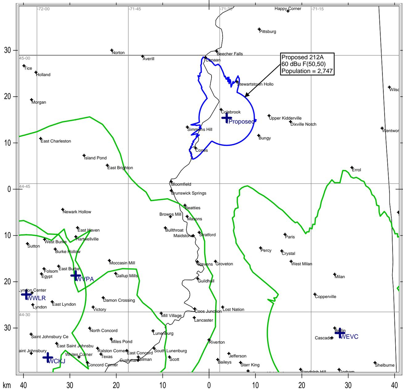
ERP = 125 Watts - Antenna HAAT = -30 Meters
