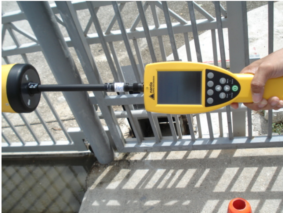
Figure 1 - Narda Meter Model NBM-550 with Shaped Probe Model EA5091
