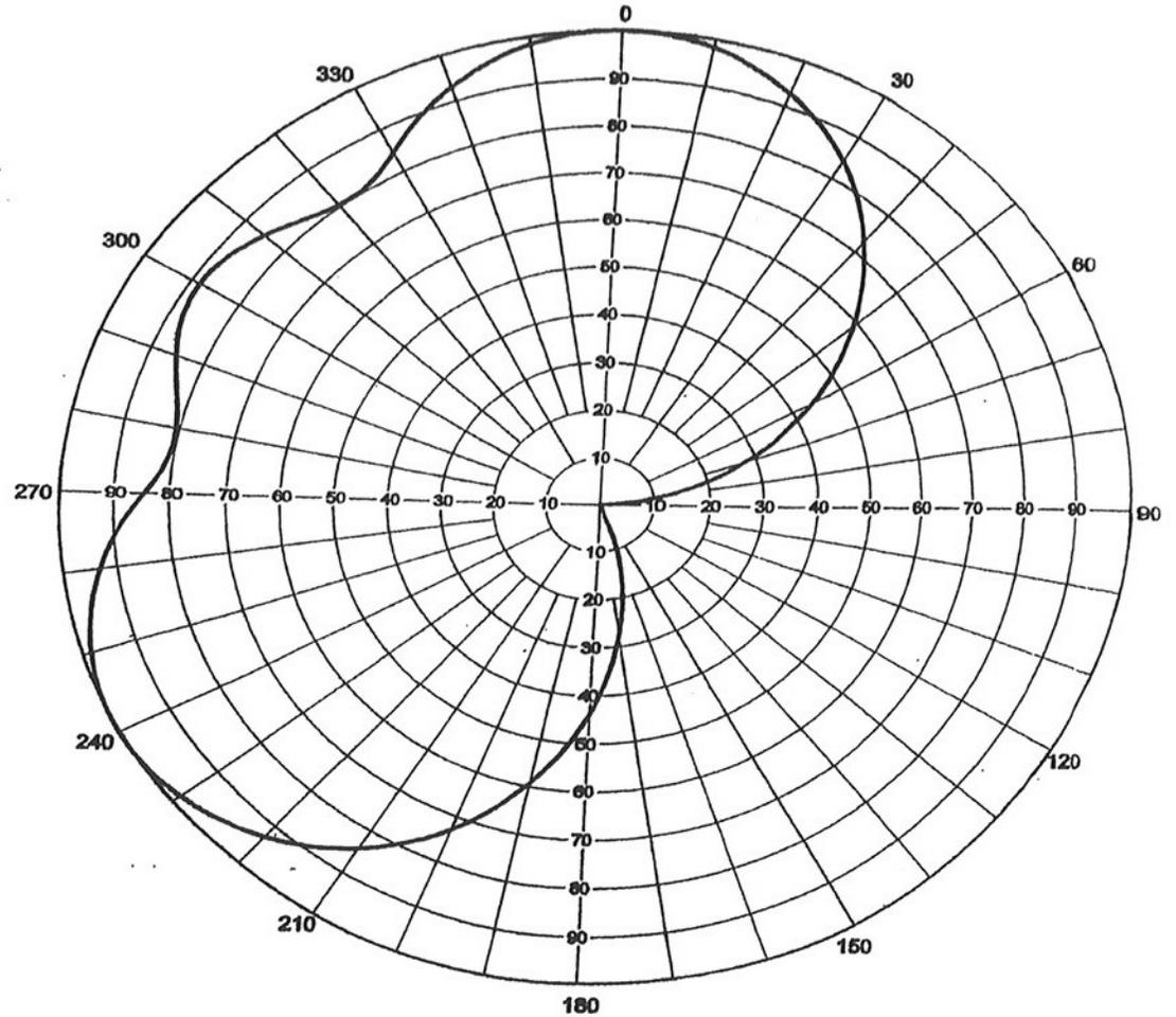
Note: Antenna will be mounted such that 0° on graph is oriented at 135°T.
