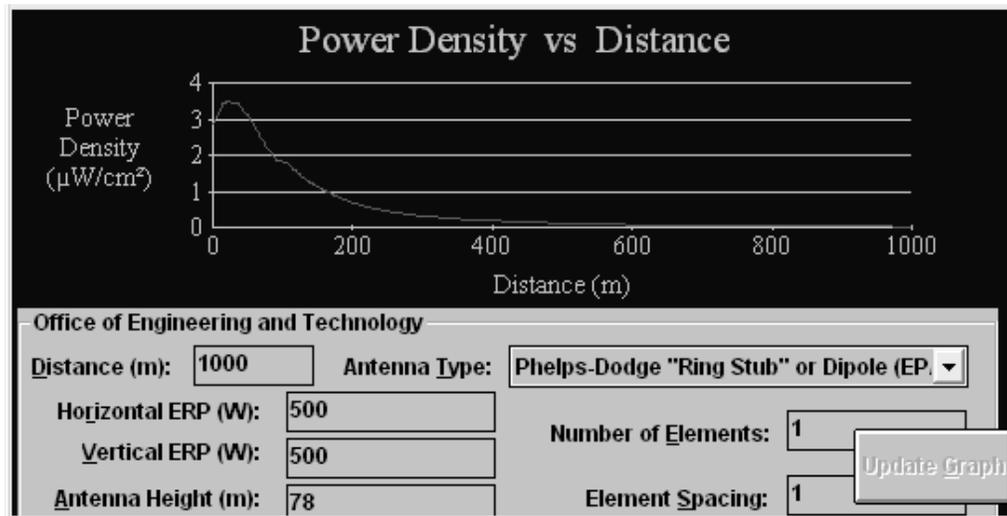
The Max Power Density was found to be 3.47952691537233  $\mu\text{W}/\text{cm}^2$  at 20 meters.
