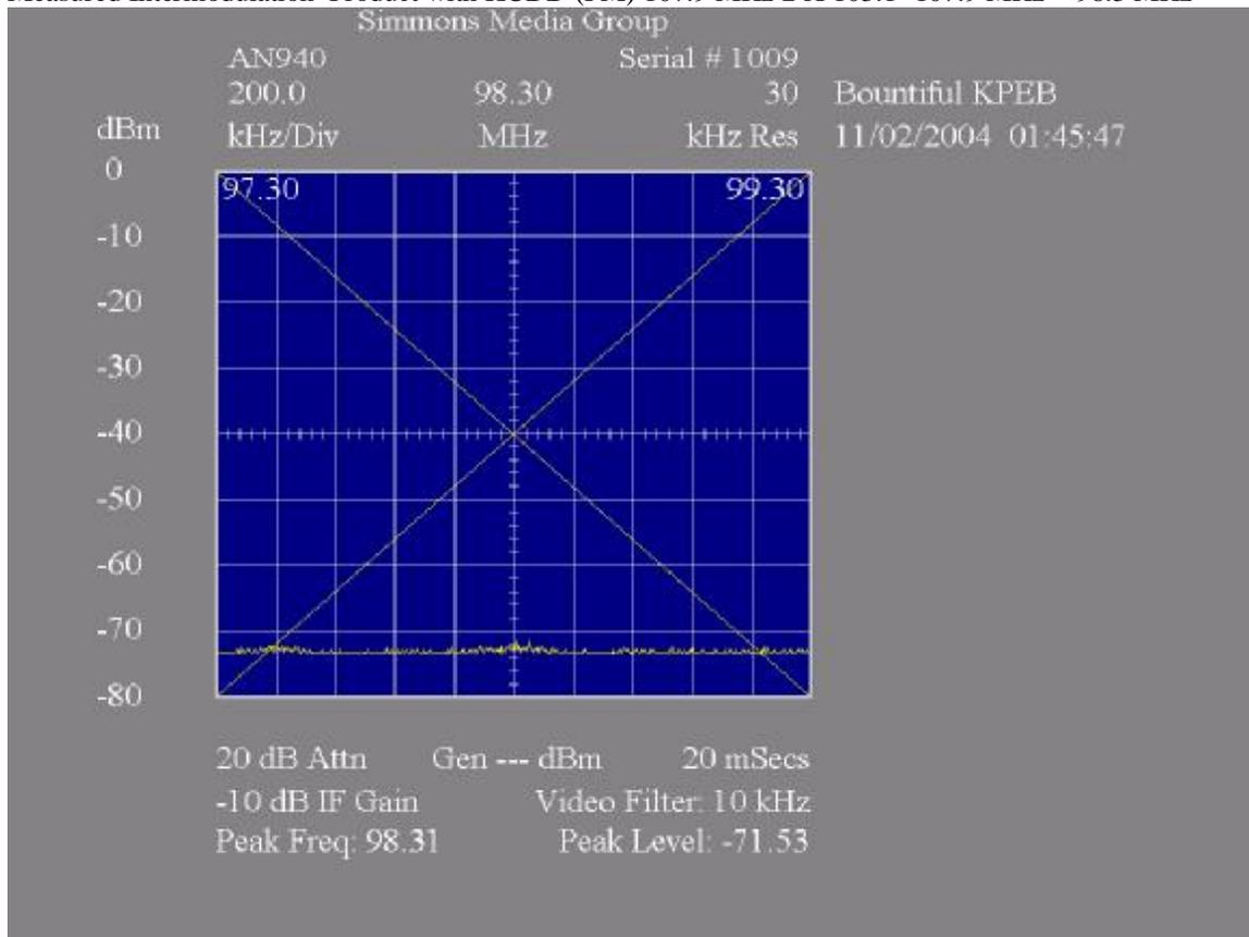
Measured Intermodulation Product with KDUT (FM) 102.3 MHz 2 X 103.1- 102.3 MHz = 103.9 MHz
