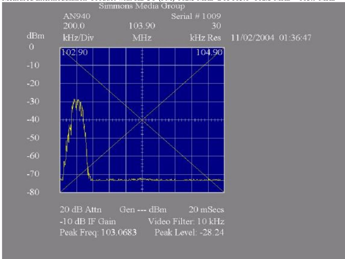
Measured Intermodulation Product with KEGA (FM) 101.5 MHz 2 X 103.1- 101.5 MHz = 104.7 MHz
