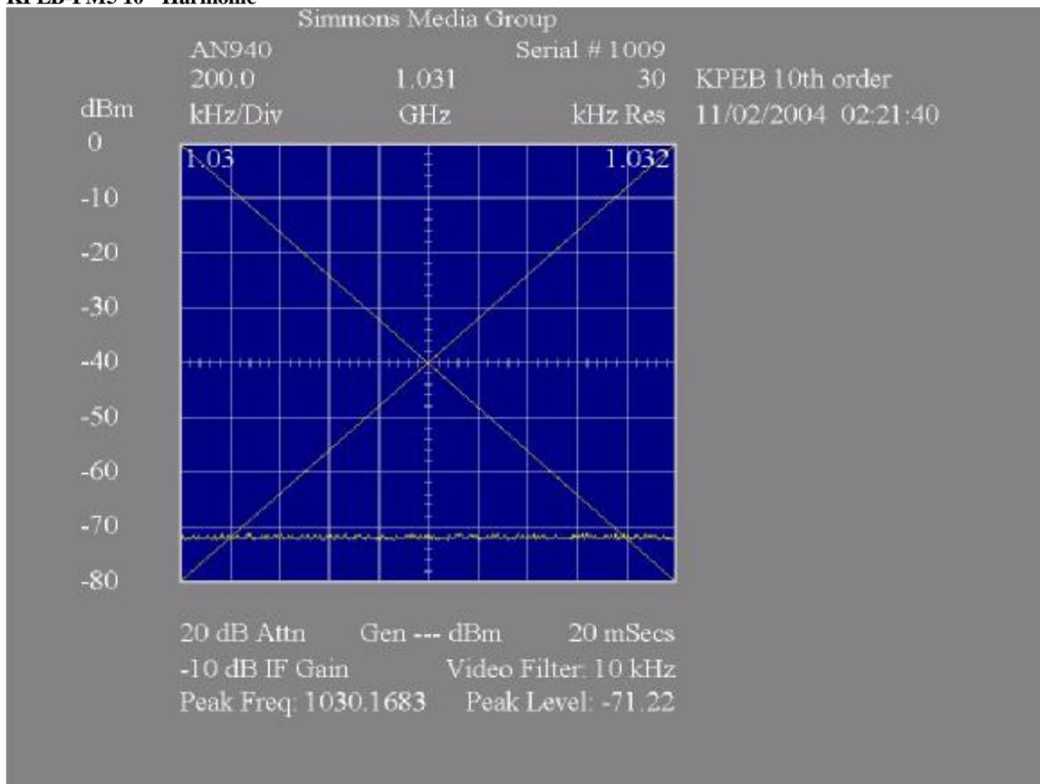
**Measured Intermodulation Product with KUDD (FM) 107.9 MHz 2 X 103.1- 107.9 MHz = 98.3 MHz**
