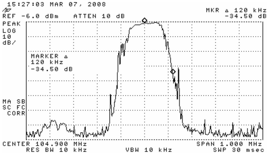
Measurement of 120KHz to 240KHz emissions Part 73.317(b) the passing condition is any measured value at or below -25dBc.
