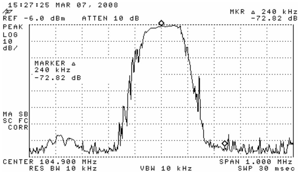
Measurement of 240KHz to 600KHz emissions Part 73.317(c) the passing condition is any measured value at or below  $-35\text{dBc}$ .
