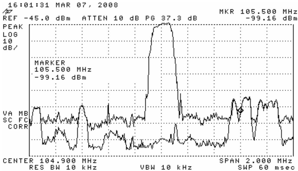
This plot shows the KRYE-FM carrier in the center with a second trace also captured and “held in memory” to measure when the KRYE-FM transmitter is turned off. If the captured trace does not change with the change of KRYE-FM, one can conclude that they are not from the transmitter.
