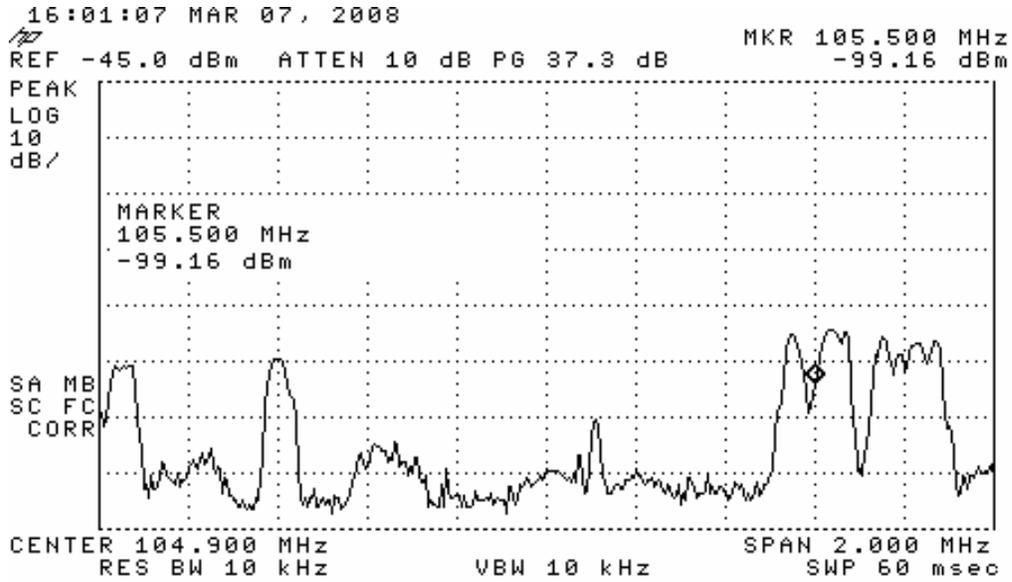
This plot shows an FM carrier that is 600KHz above KRYE-FM that prevents the 73.317(d) measurement.
