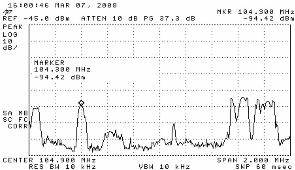
This plot shows an FM carrier that is 600KHz below KRYE-FM that prevents the 73.317(d) measurement.
