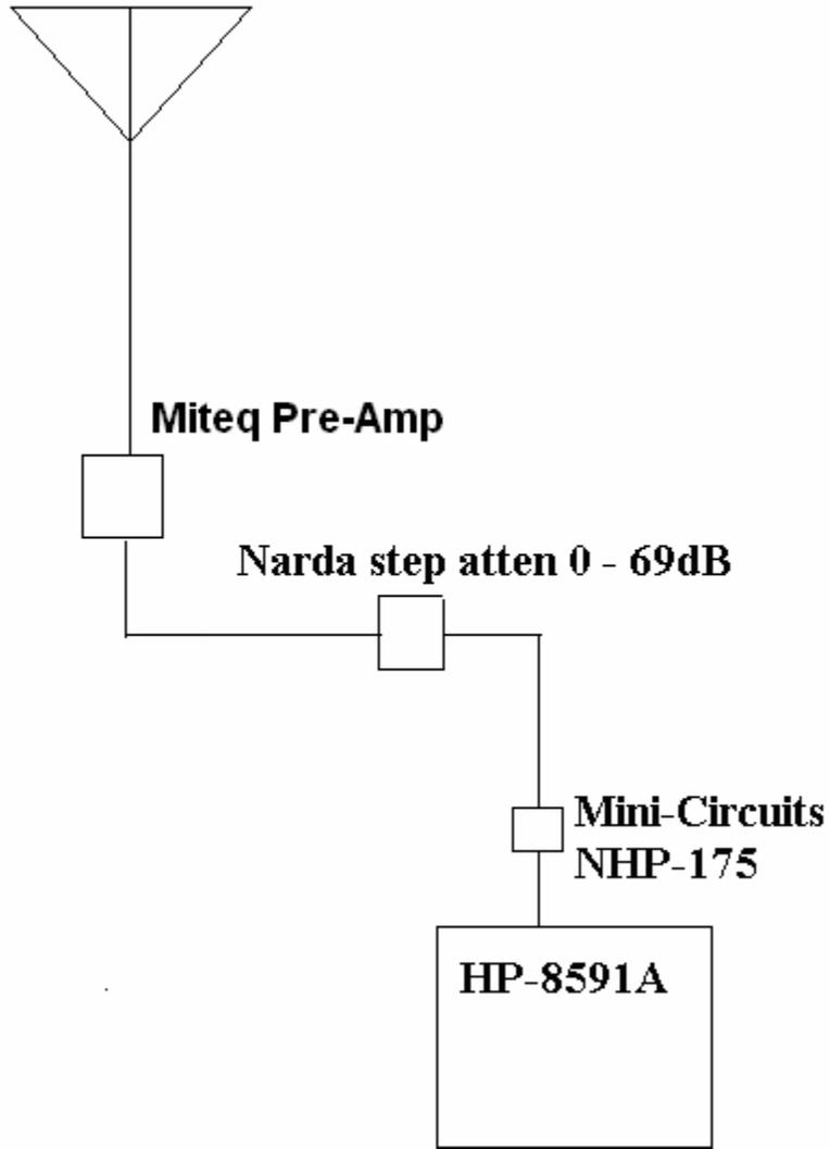
Above is a block diagram of the test jig, or equipment configuration during the measurements of the transmitter, near Rye Colorado.
