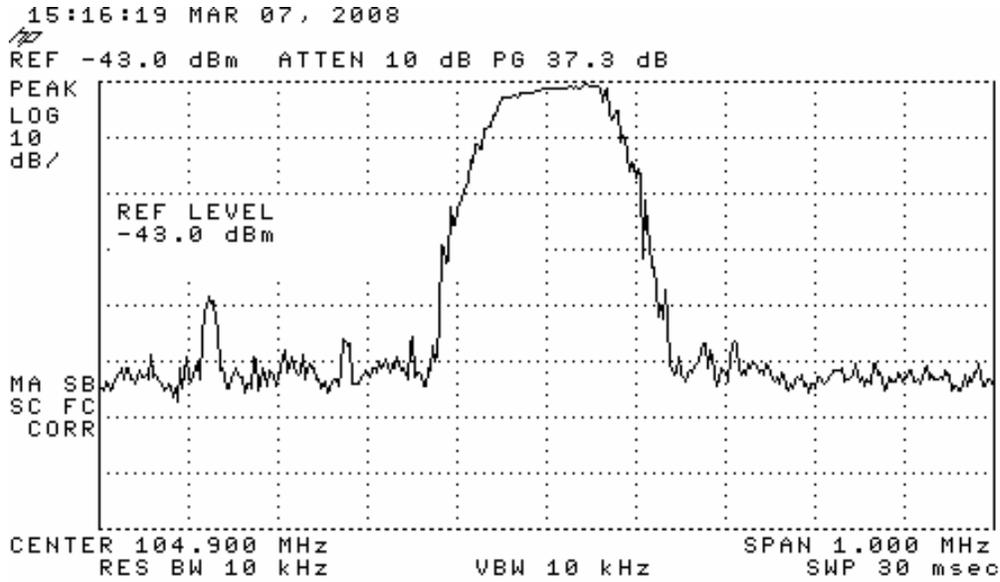
Above is the peak-hold of KRYE (104.9 MHz). This was verification that the amplitude was adjusted correctly with the Narda step attenuator so that a reference point for the remaining measurements relative to the carrier.
